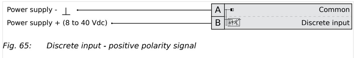
Fig. 65: Discrete input - positive polarity signal
