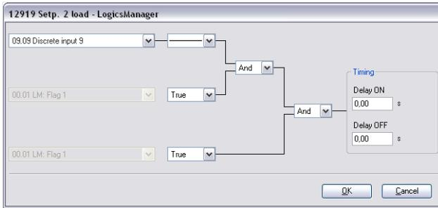
Fig. 232: LogicsManager function "Setp. 2 load"
