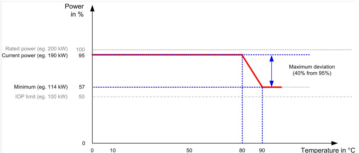
Fig. 291: Derating: Islanded parallel operation
