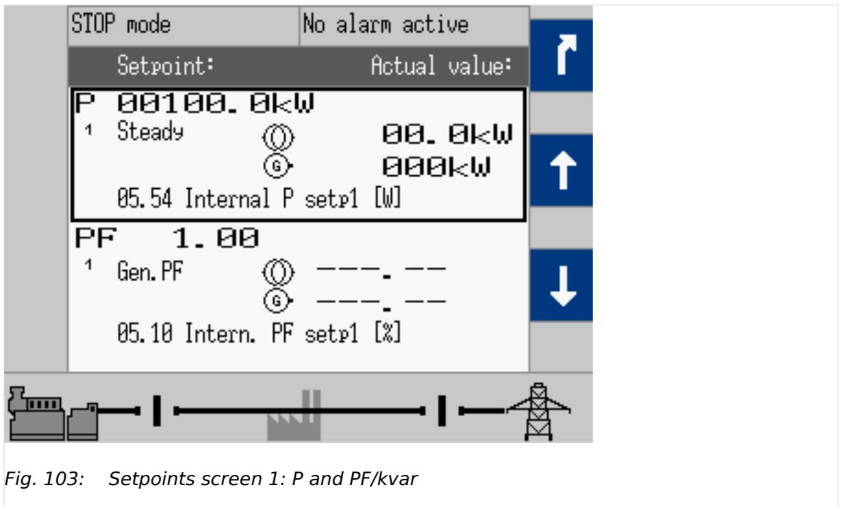
Fig. 103: Setpoints screen 1: P and PF/kvar
