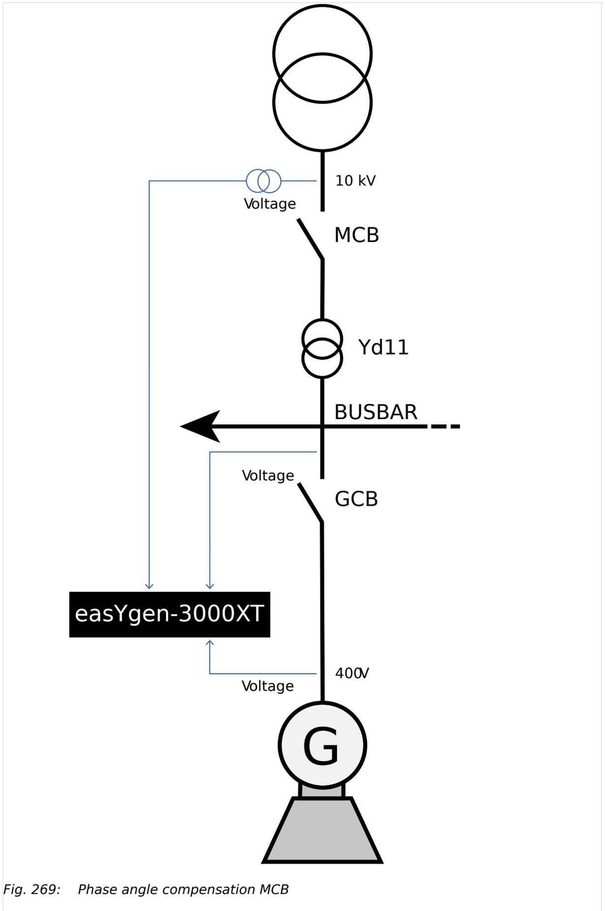
Fig. 269: Phase angle compensation MCB
