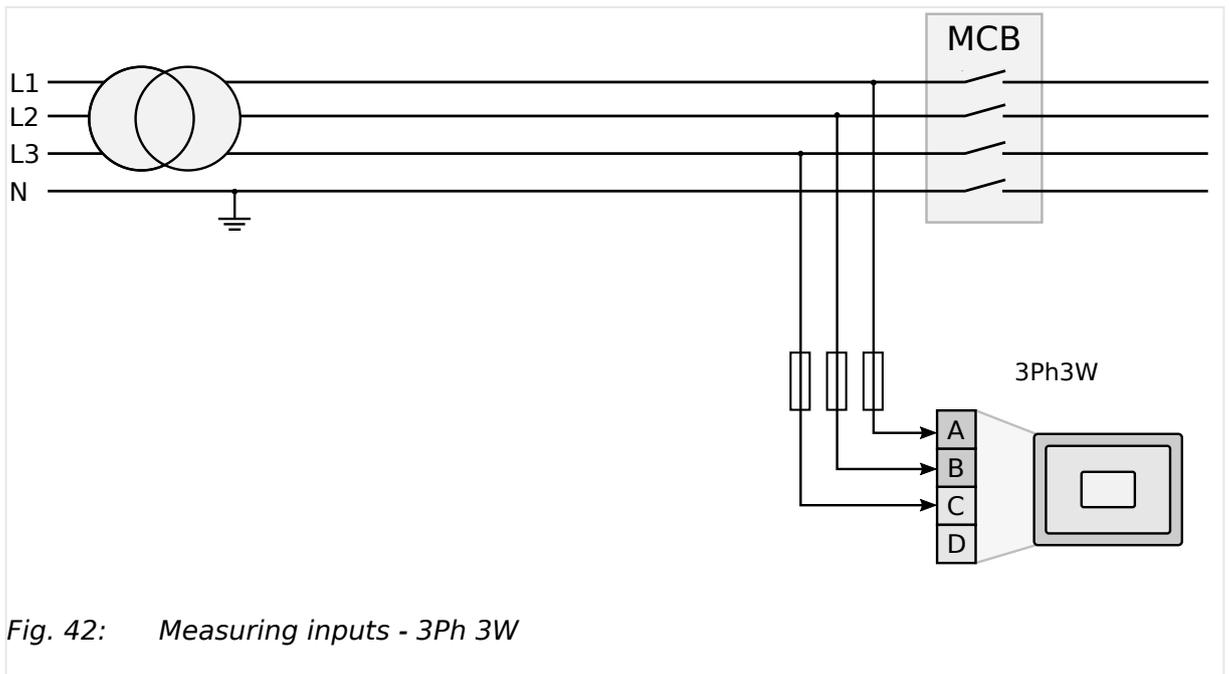
Fig. 42: Measuring inputs - 3Ph 3W
