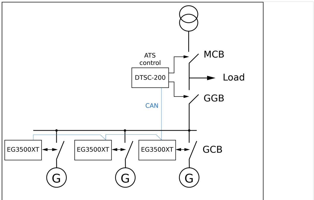
Fig. 288: Example of an application with parameter 9066 "Predicted load source" is configured as "External". Additionally, there is a hardwired inhibit signal from easYgens to the ATS".
