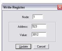
Fig. 329: Write register - acknowledge alarm message
