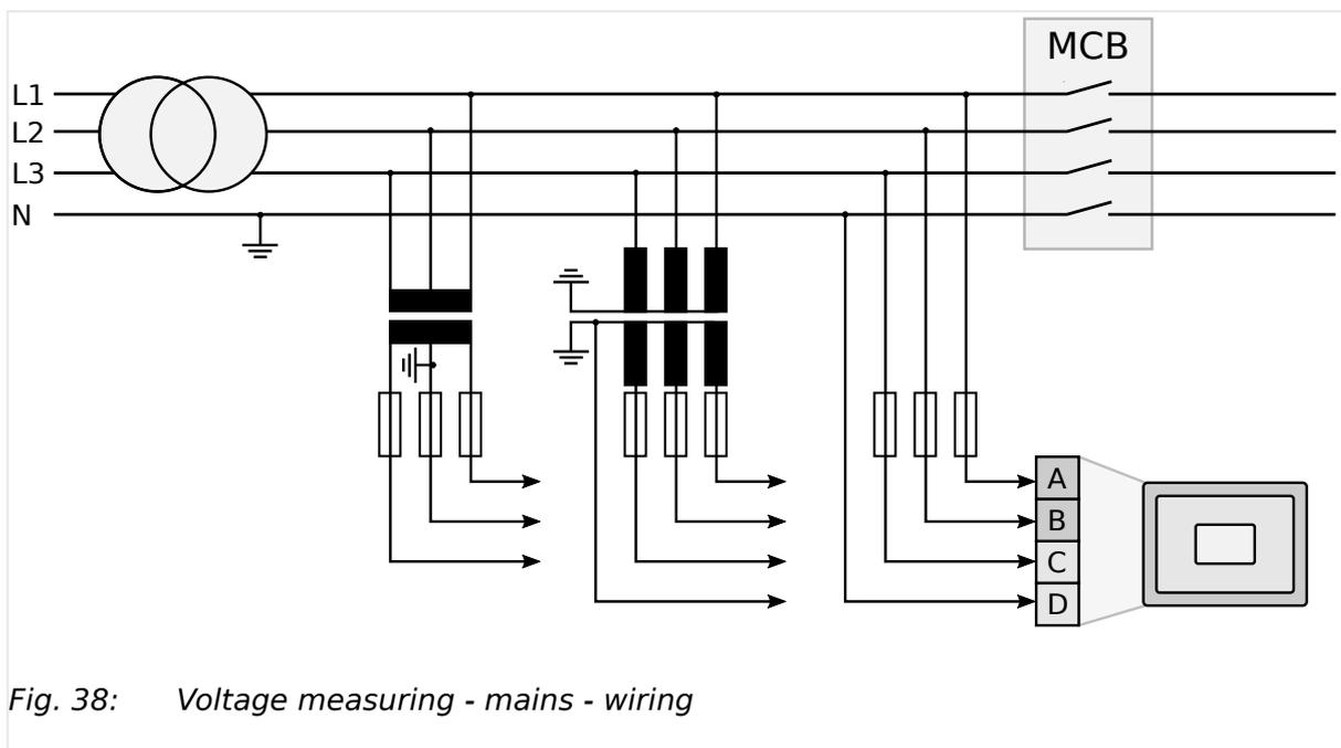
Fig. 38: Voltage measuring - mains - wiring
