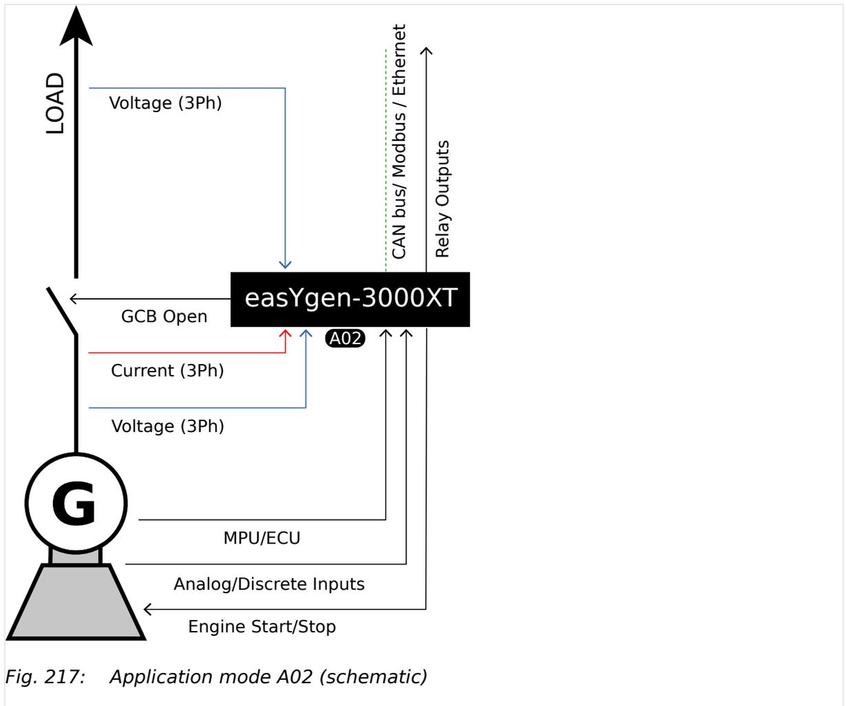
Fig. 217: Application mode A02 (schematic)
