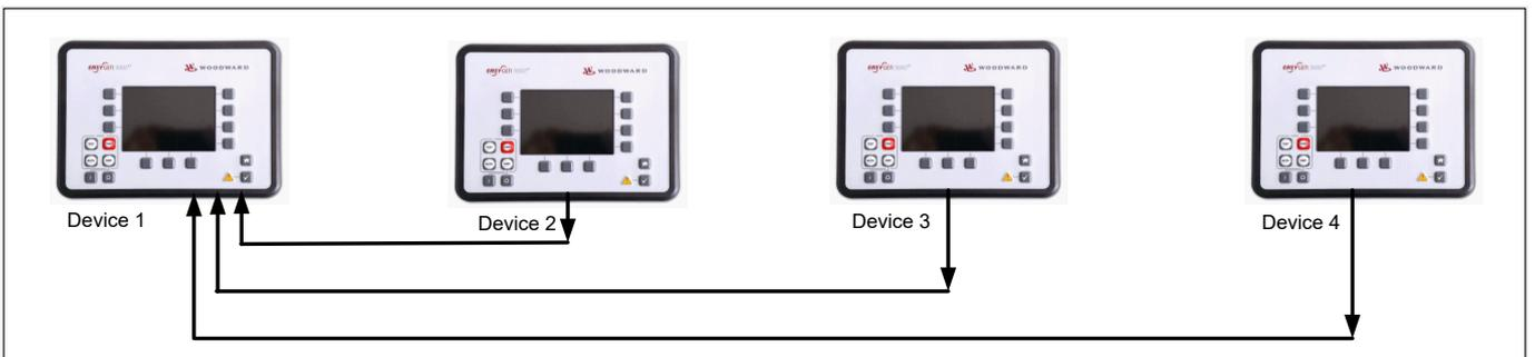
Fig. 228: Device 1 receives data from device 2, 3 and 4
