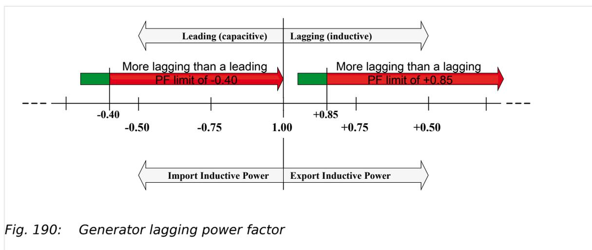
Fig. 190: Generator lagging power factor
