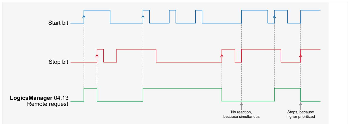
Fig. 361: Remote control - start/stop priority
