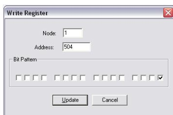
Fig. 293: Modbus - write register - start request
