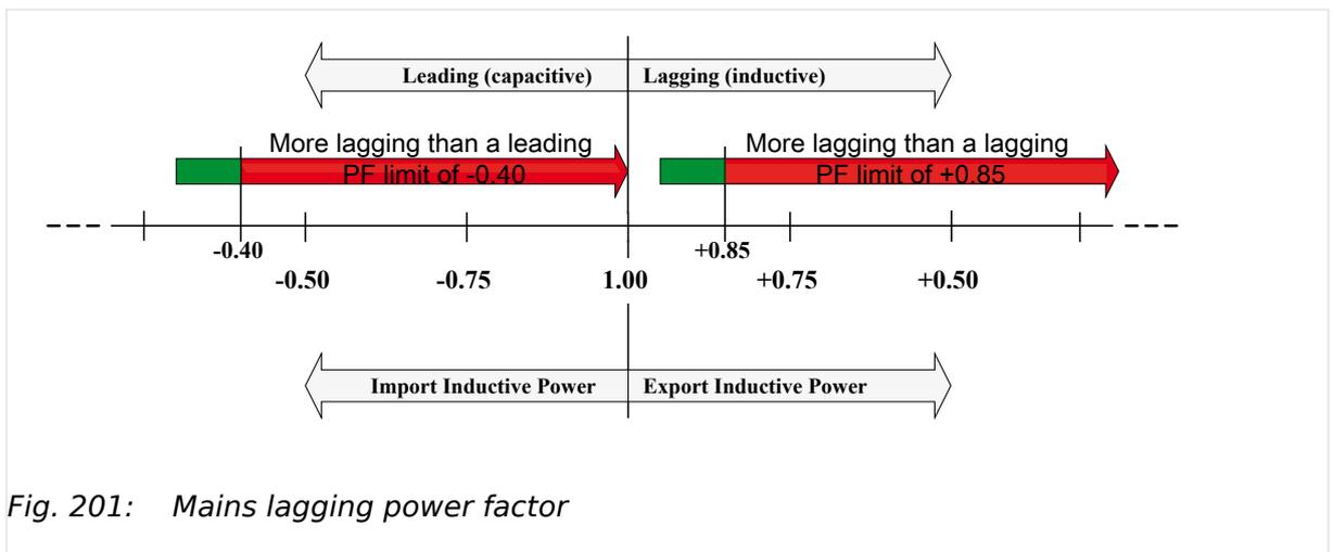
Fig. 201: Mains lagging power factor
