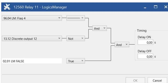
Fig. 236: LogicsManager function "Relay 11"
