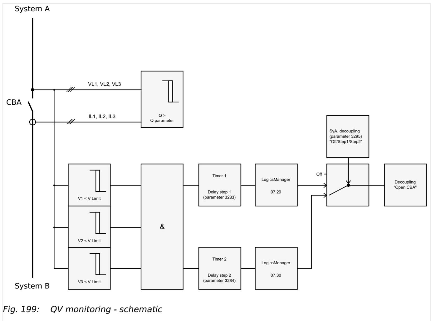
Fig. 199: QV monitoring - schematic
