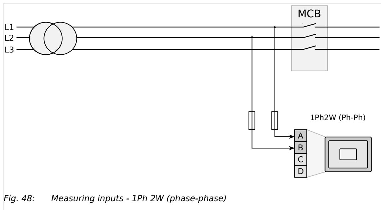
Fig. 48: Measuring inputs - 1Ph 2W (phase-phase)
