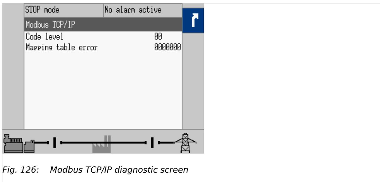
Fig. 126: Modbus TCP/IP diagnostic screen
