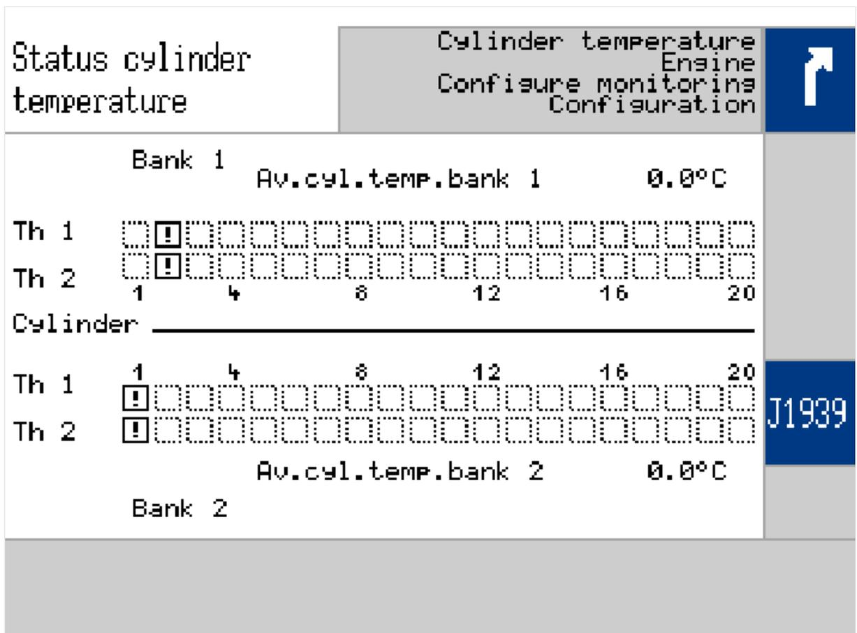
Fig. 196: Cylinder temperature screen
