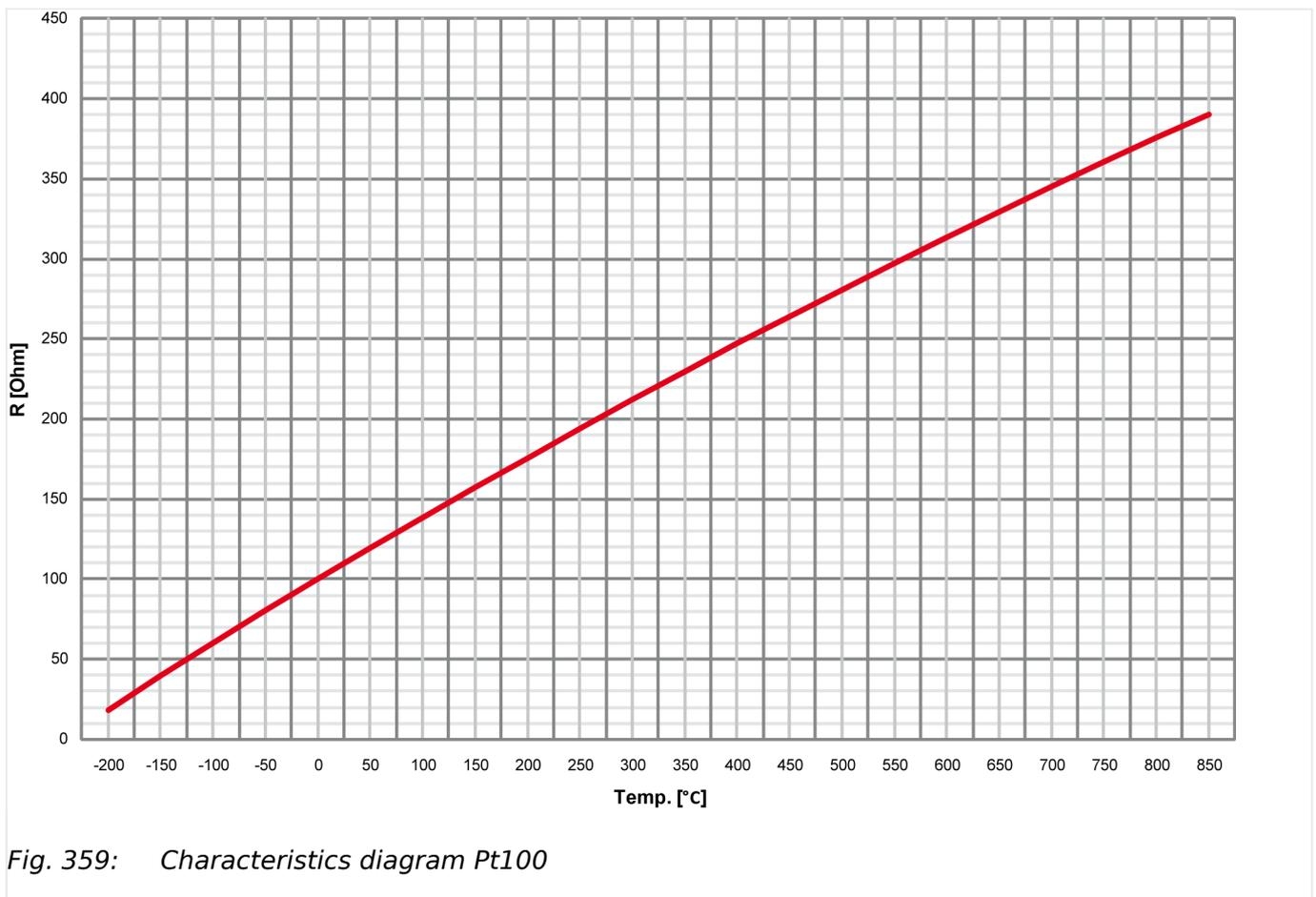
Fig. 359: Characteristics diagram Pt100
