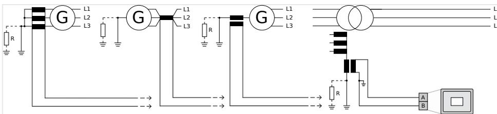
Fig. 59: Current measuring - ground current - wiring
