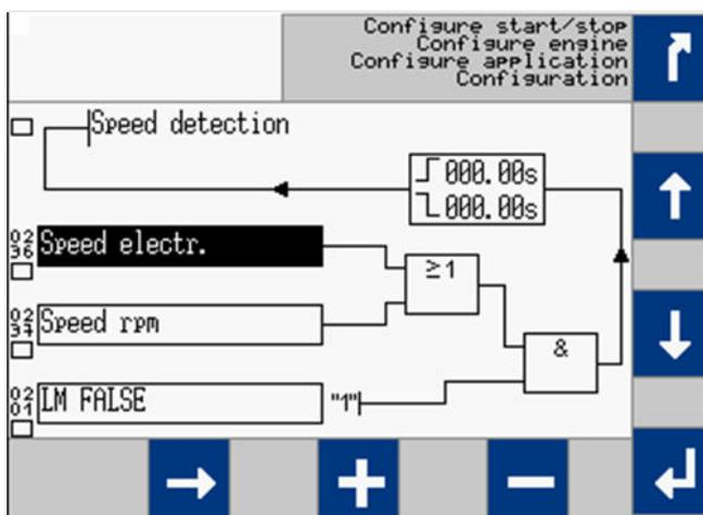
*Fig. 150: LogicsManager for detecting speed*
