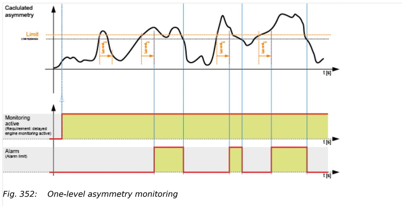
Fig. 352: One-level asymmetry monitoring
