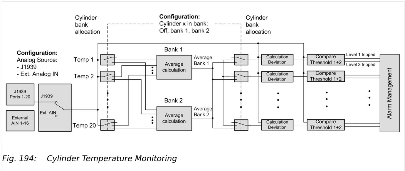
Fig. 194: Cylinder Temperature Monitoring
