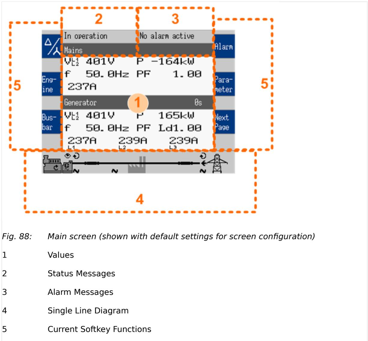
Fig. 88: Main screen (shown with default settings for screen configuration)
