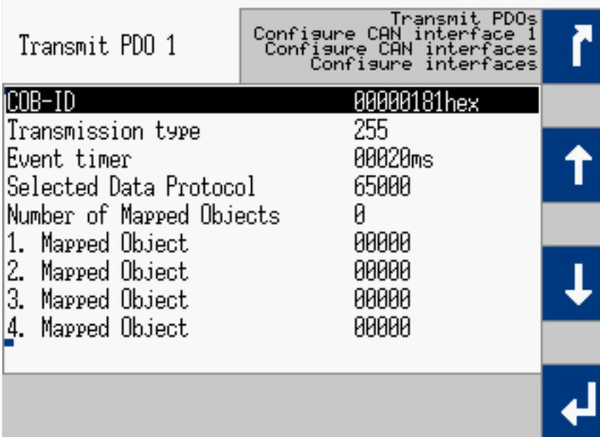
Fig. 250: TPDO configuration for IKD 1 (example HMI)
