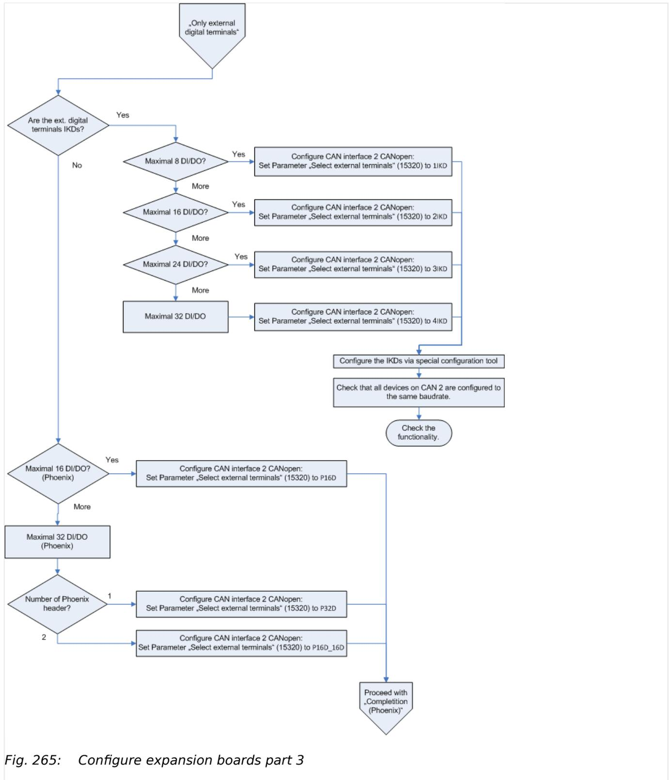
Fig. 265: Configure expansion boards part 3
