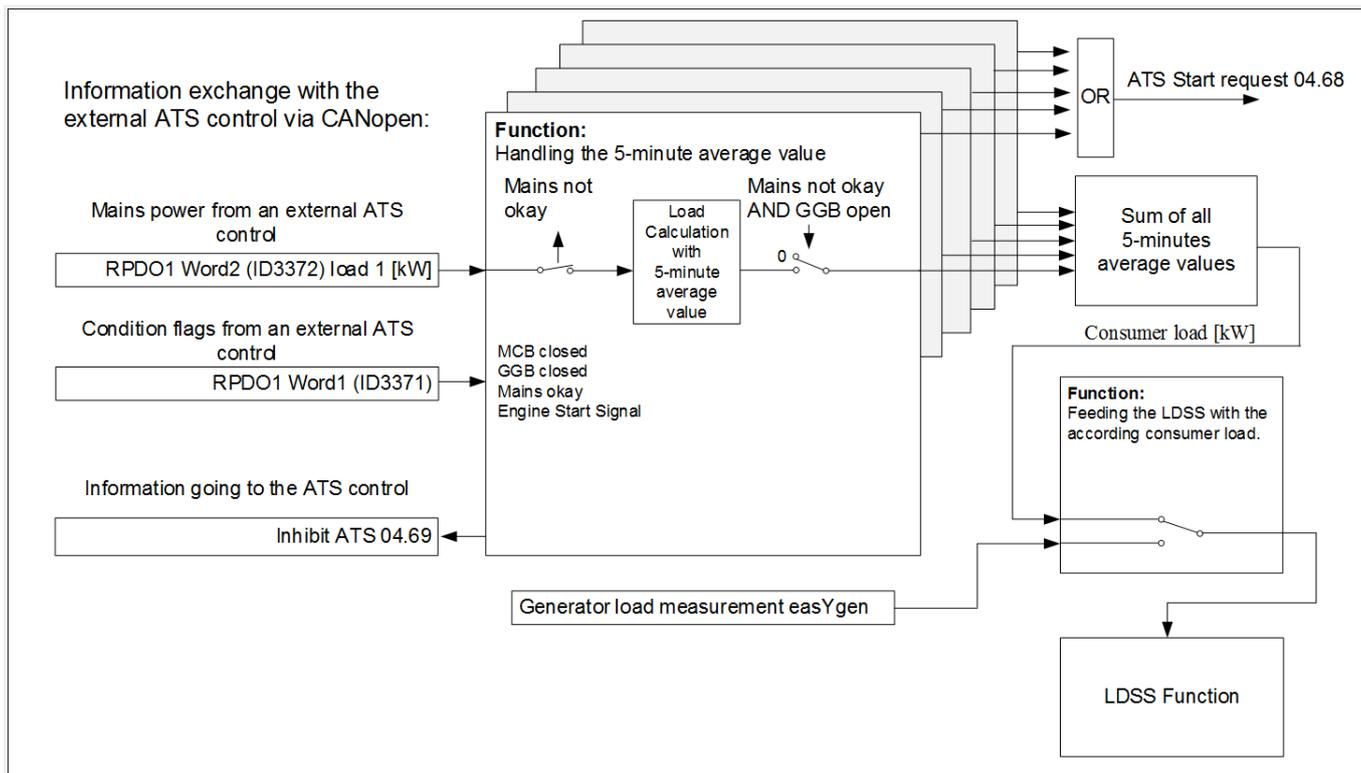
Fig. 287: The principle of the LDSS PL in external source mode
