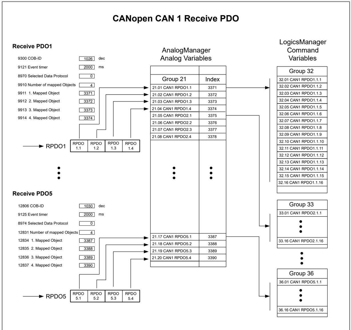
Fig. 363: Example of a CAN 1 RPDO configuration for interconnectivity.
