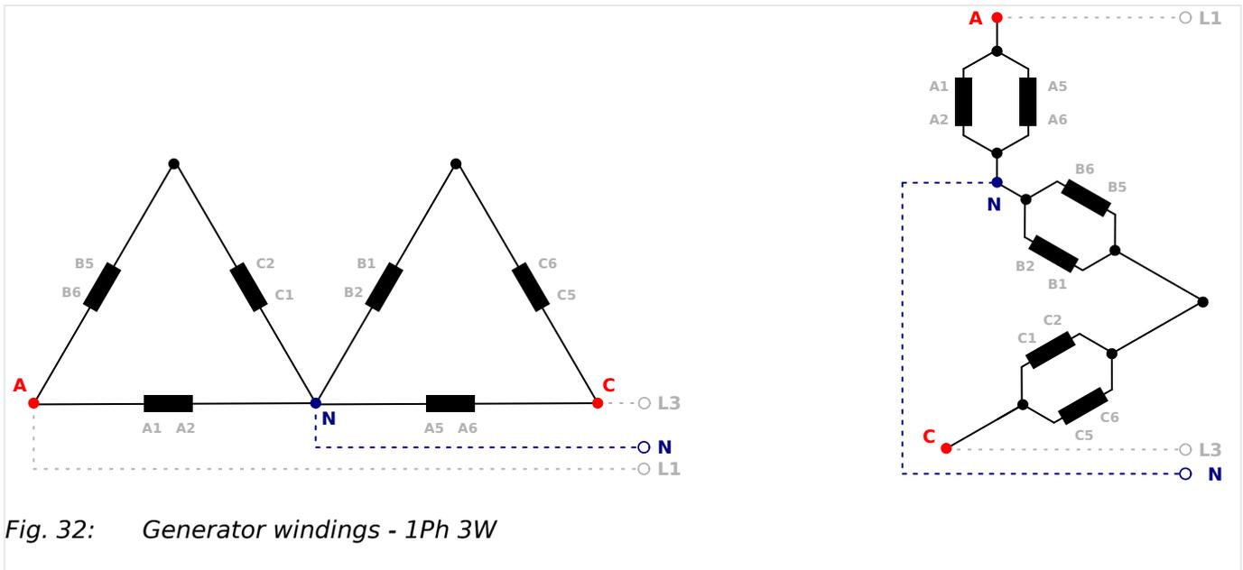
Fig. 32: Generator windings - 1Ph 3W
