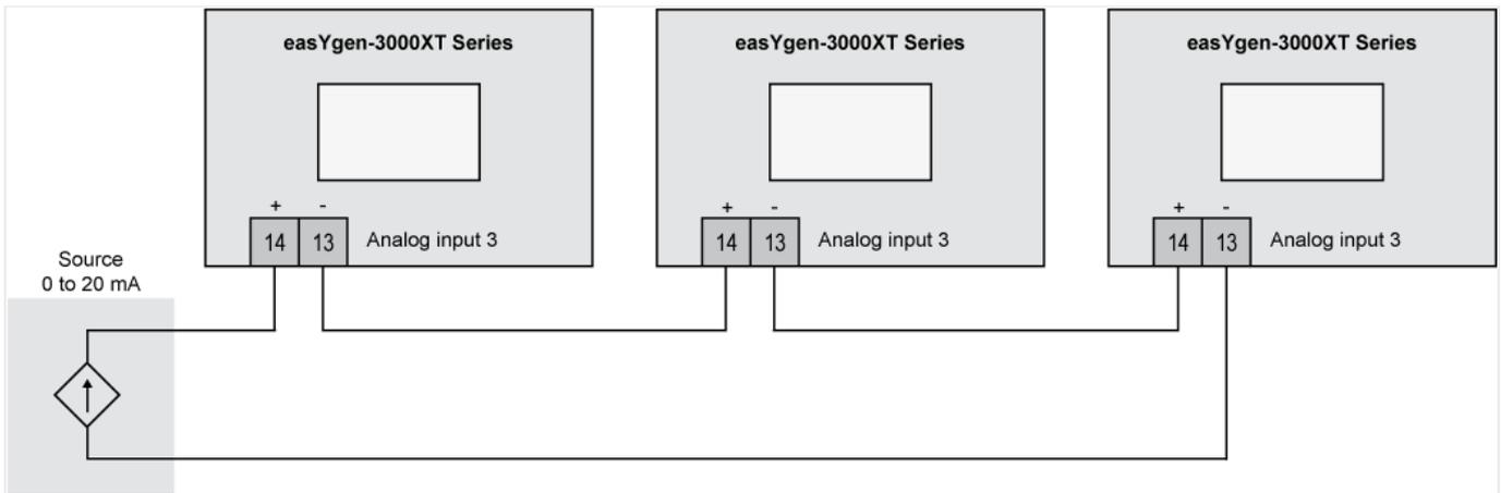
Fig. 261: Connecting analog inputs in series
