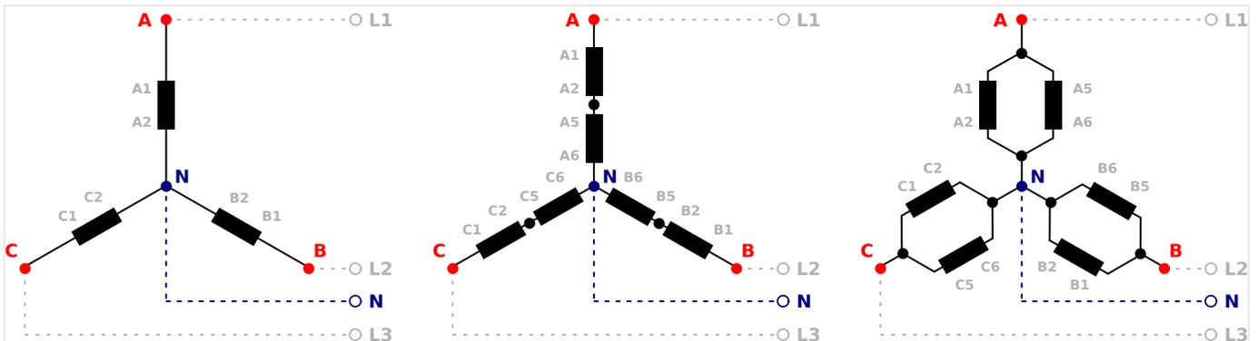
Fig. 28: Generator windings - 3Ph 4W
