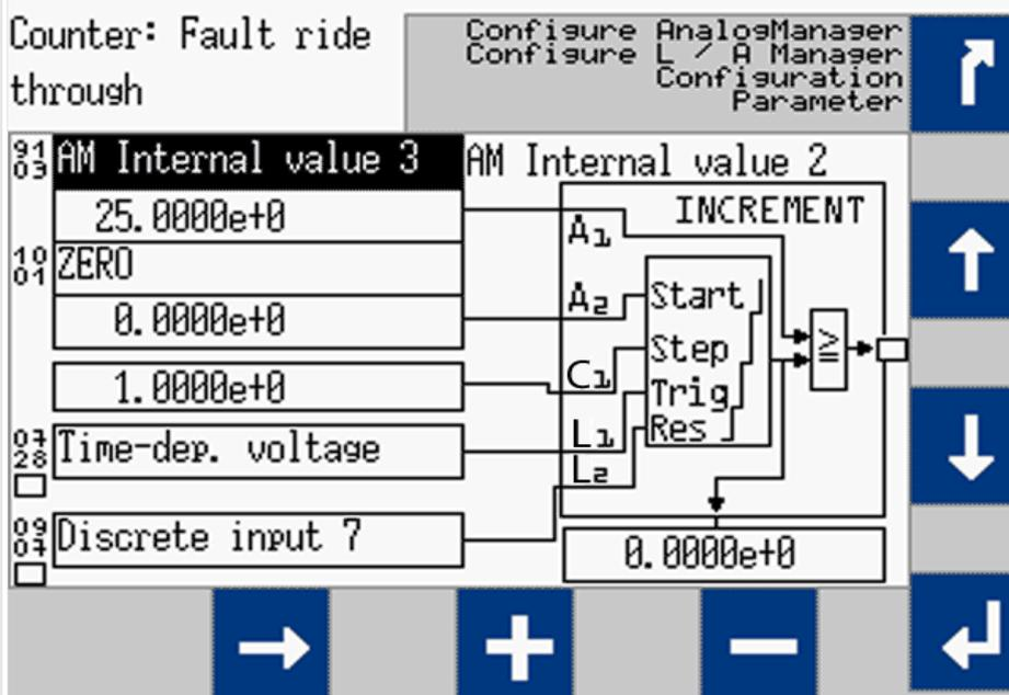
Fig. 213: screen shot HMI: AM increment sample
