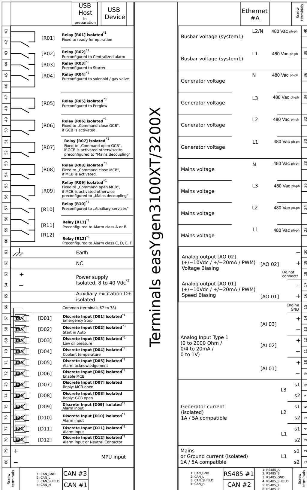
Subject to technical modifications \*1configurable via Logics Manager easYgen-3000XT Series Wiring Diagram PCB 1
