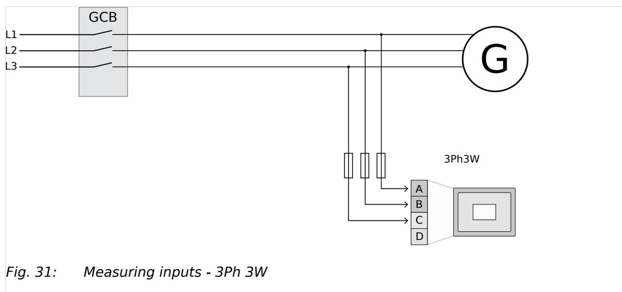
Fig. 31: Measuring inputs - 3Ph 3W
