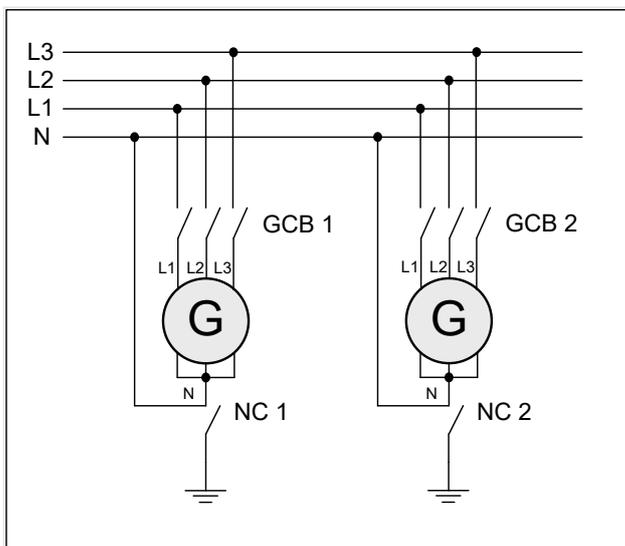
Fig. 278: Wiring neutral Interlocking: GCB 3-pole
