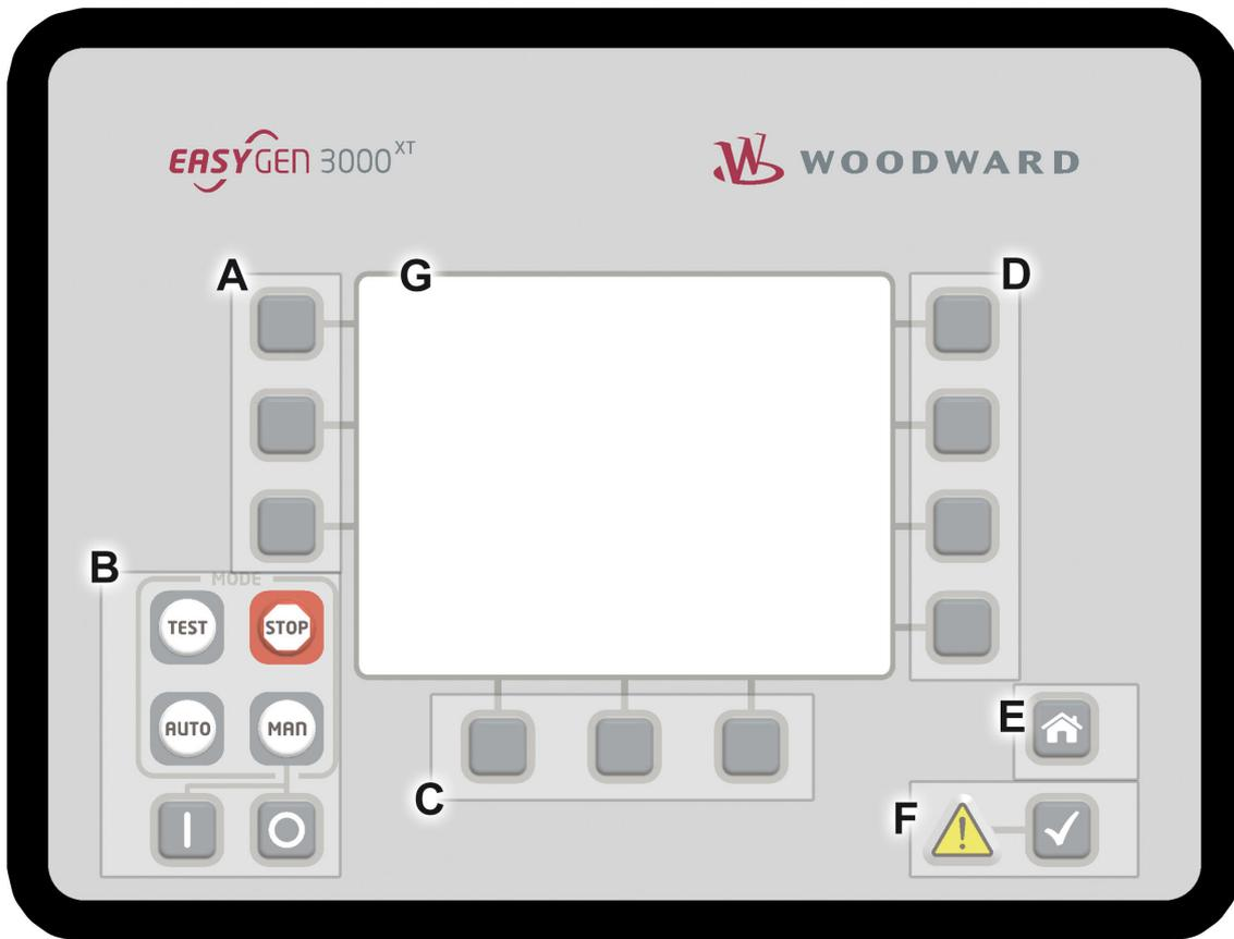
Fig. 3: Front Panel, Overview of Functional Groups of easYgen-3000XT with plastic housing
