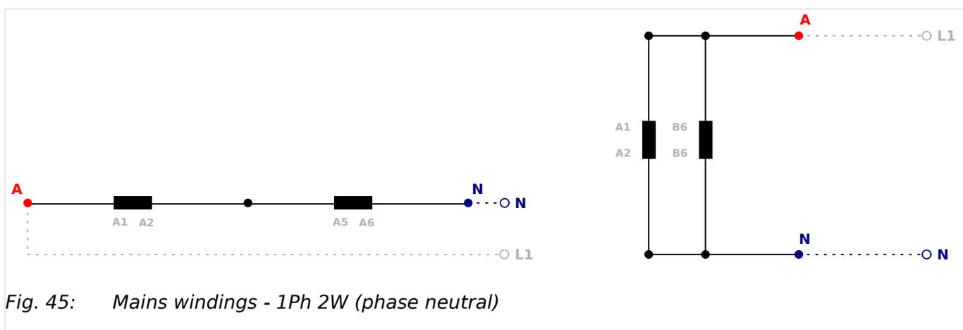
Fig. 45: Mains windings - 1Ph 2W (phase neutral)
