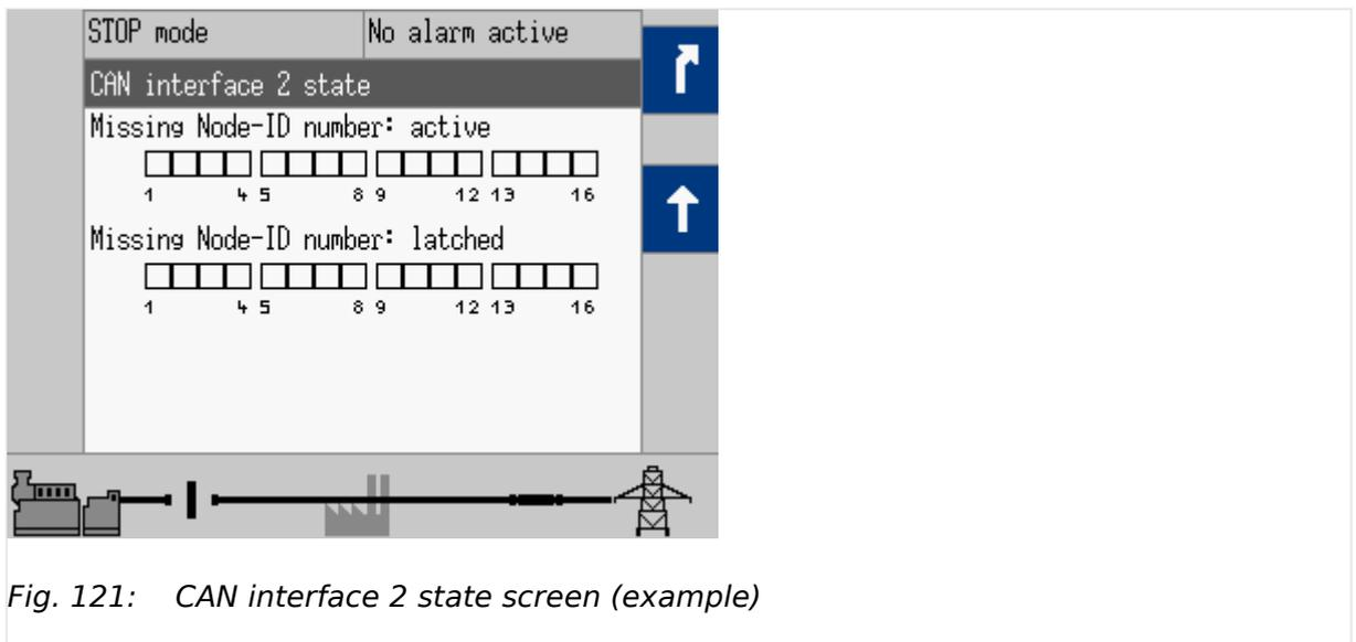
Fig. 121: CAN interface 2 state screen (example)
