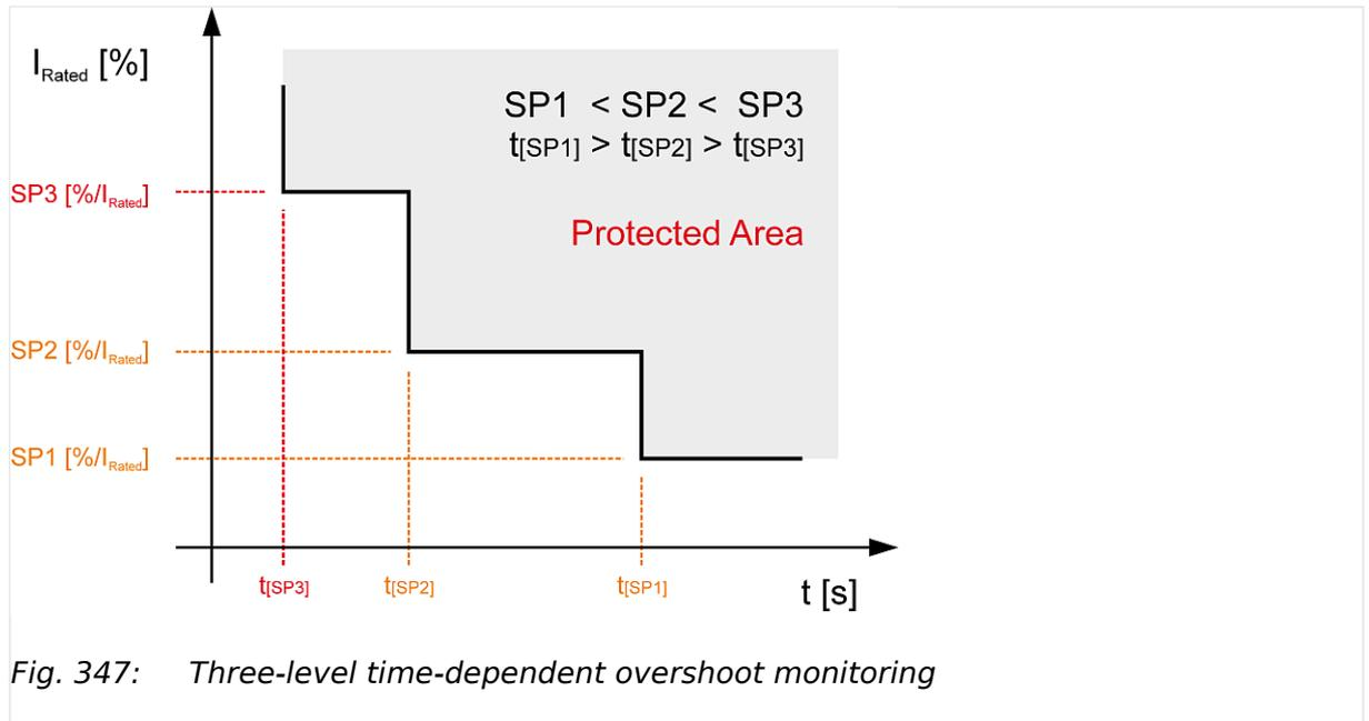
Fig. 347: Three-level time-dependent overshoot monitoring
