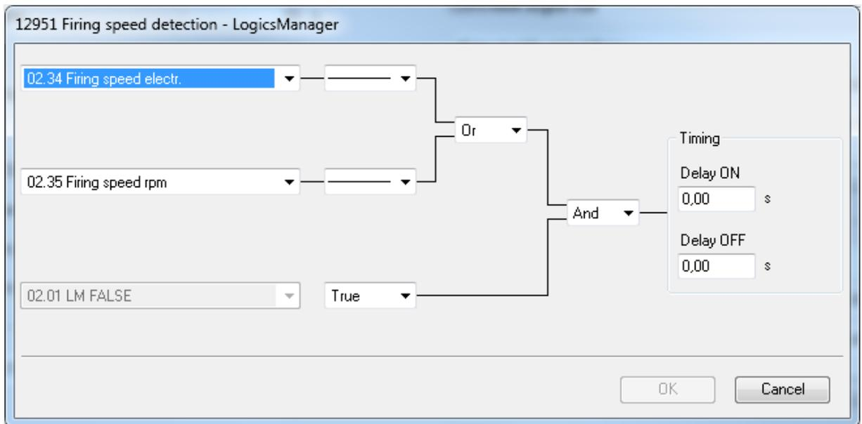
Fig. 270: LogicsManager function "Firing speed detection"
