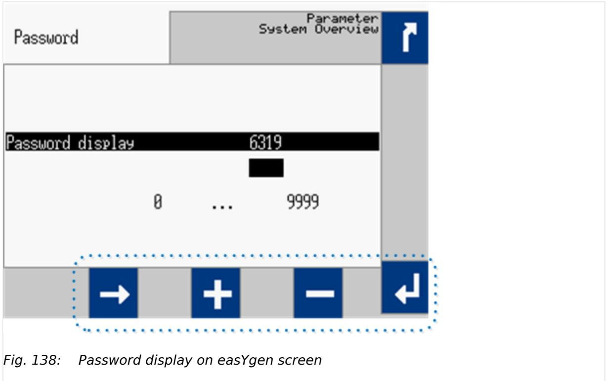
Fig. 138: Password display on easYgen screen
