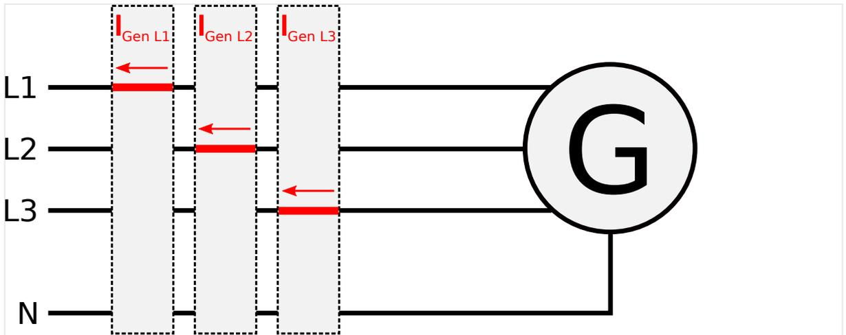
Fig. 55: Current measuring - generator, L1 L2 L3
