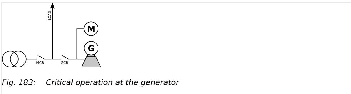
Fig. 183: Critical operation at the generator
