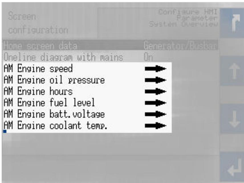
Fig. 90: AnalogManagers for "Engine" values at Home Screen
