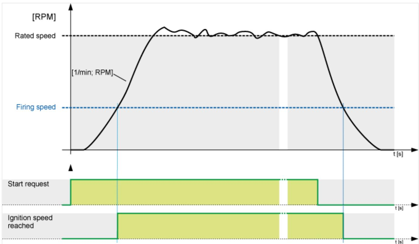
Fig. 151: Engine - firing speed
