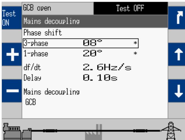
Fig. 114: Mains decoupling screen 3
