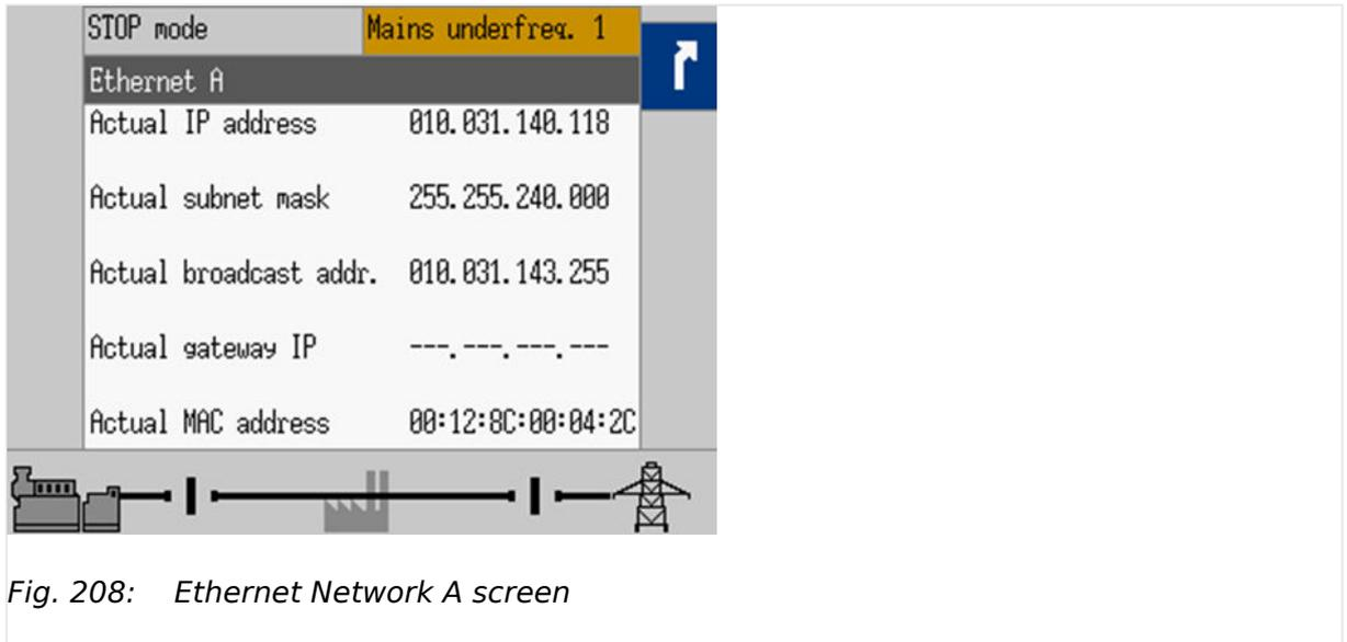
Fig. 208: Ethernet Network A screen
