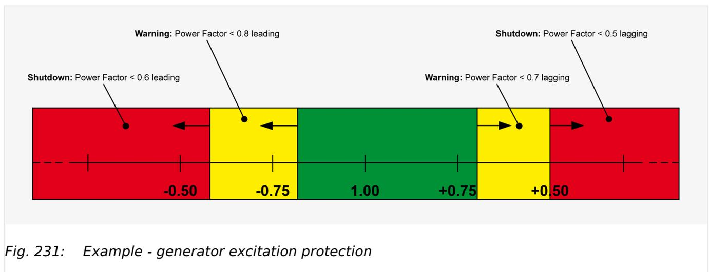
↳ Fig. 231 shows a typical power factor (generator excitation) protection range, where the desired range of operation (green area) is from 0.7 lagging (inductive) to 0.8 leading (capacitive).
