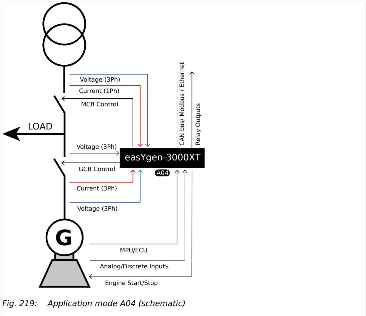
Fig. 219: Application mode A04 (schematic)
