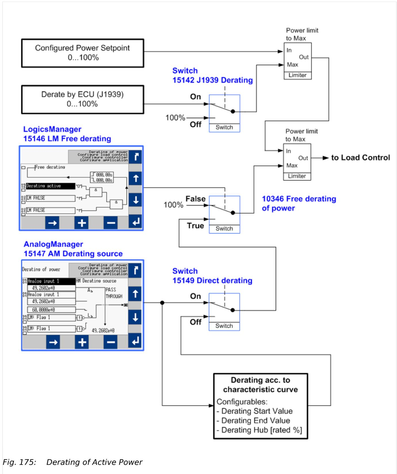
Fig. 175: Derating of Active Power
