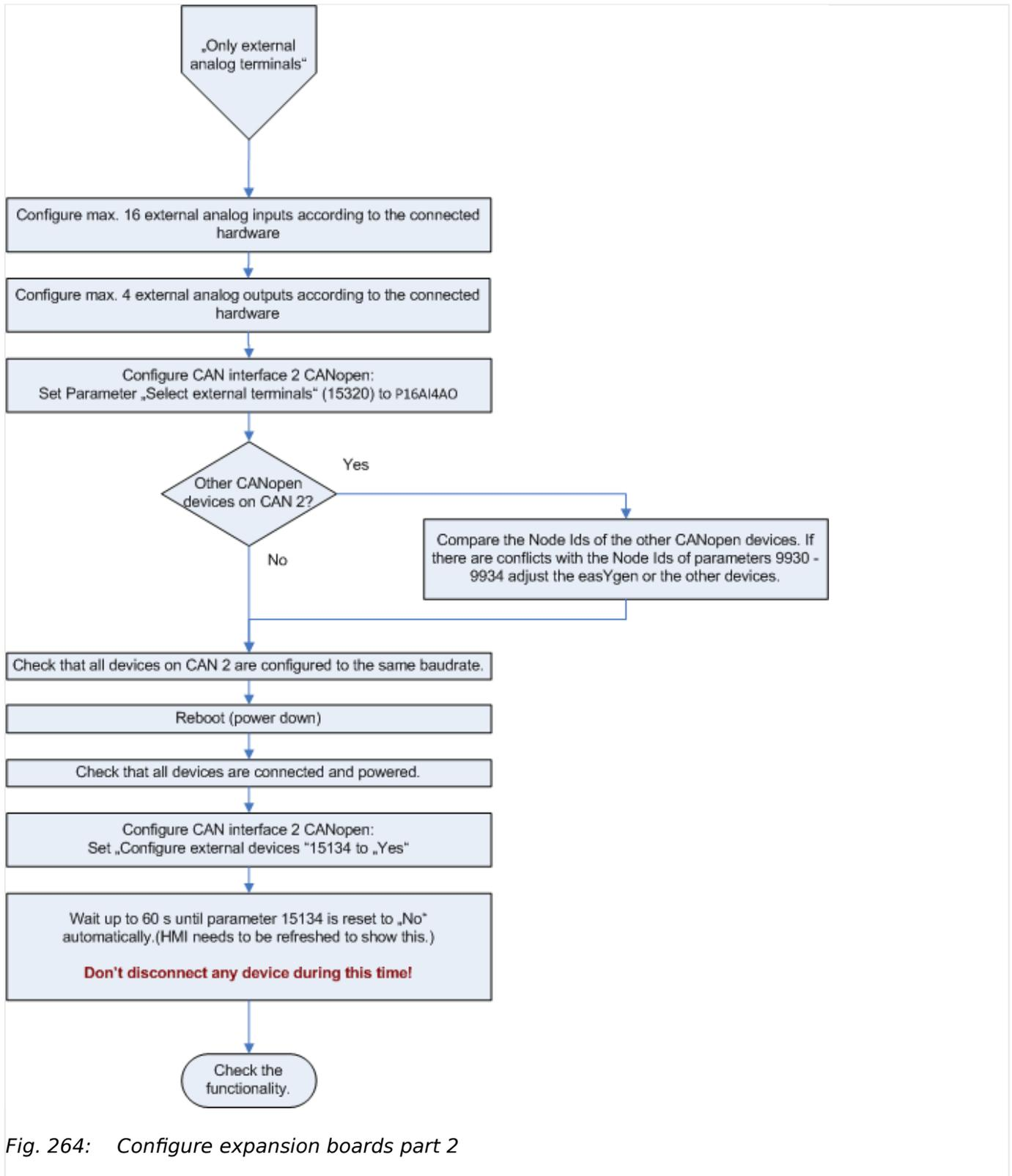
Fig. 264: Configure expansion boards part 2
