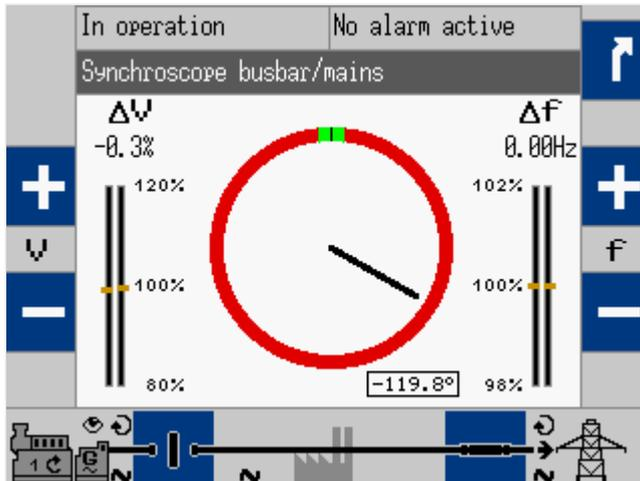
Fig. 108: Synchroscope screen (example)
