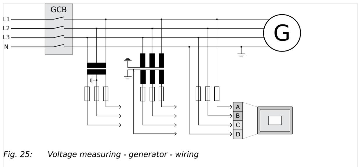
Fig. 25: Voltage measuring - generator - wiring
