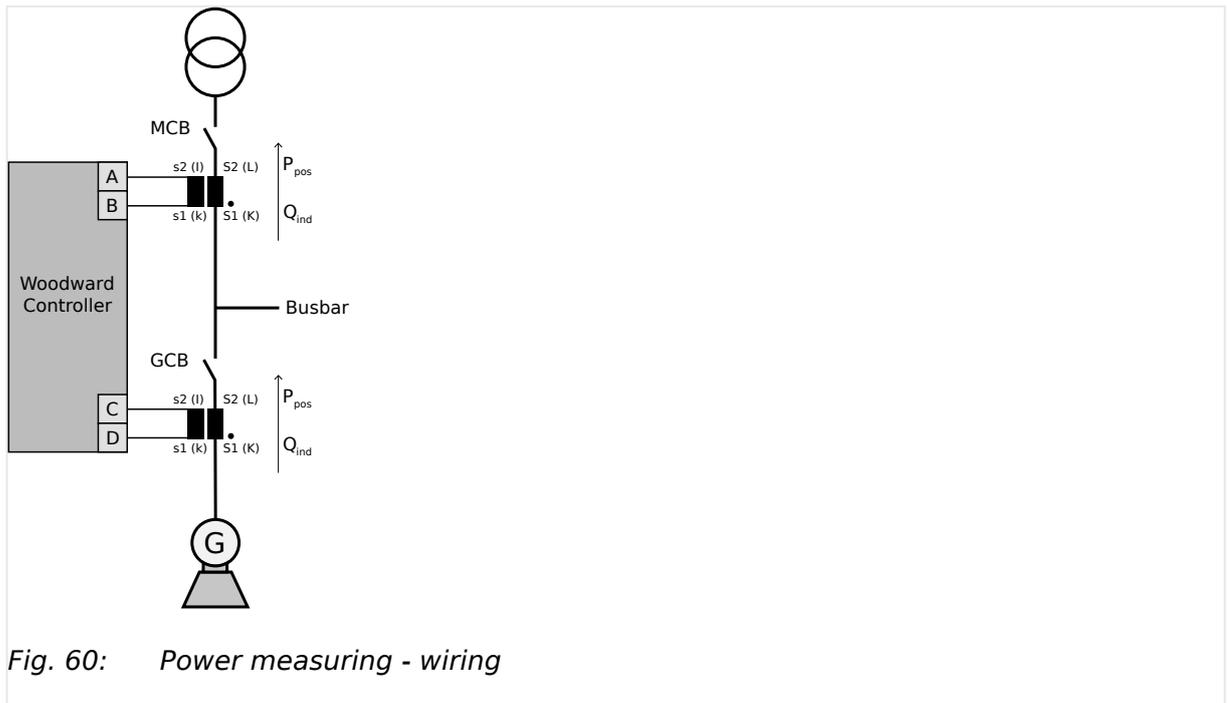
Fig. 60: Power measuring - wiring
