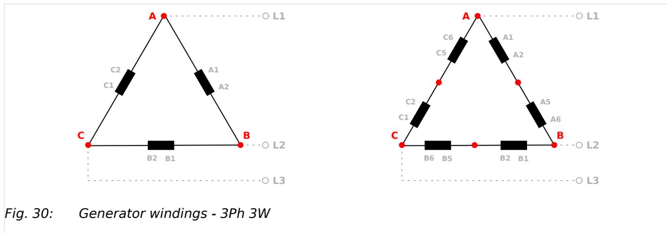
Fig. 30: Generator windings - 3Ph 3W
