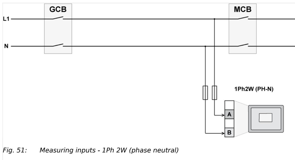
Fig. 51: Measuring inputs - 1Ph 2W (phase neutral)
