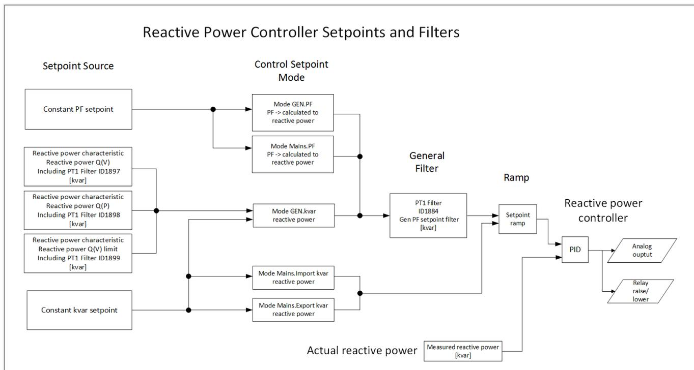
Fig. 167: The allocation of reactive power setpoints and their filters
