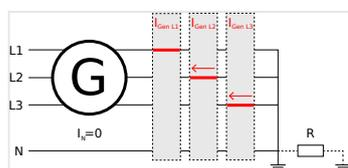
Fig. 192: Generator ground fault - schematic
