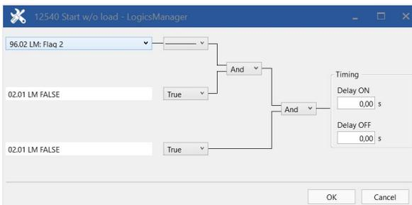
Fig. 246: LogicsManager function "Start without load"
