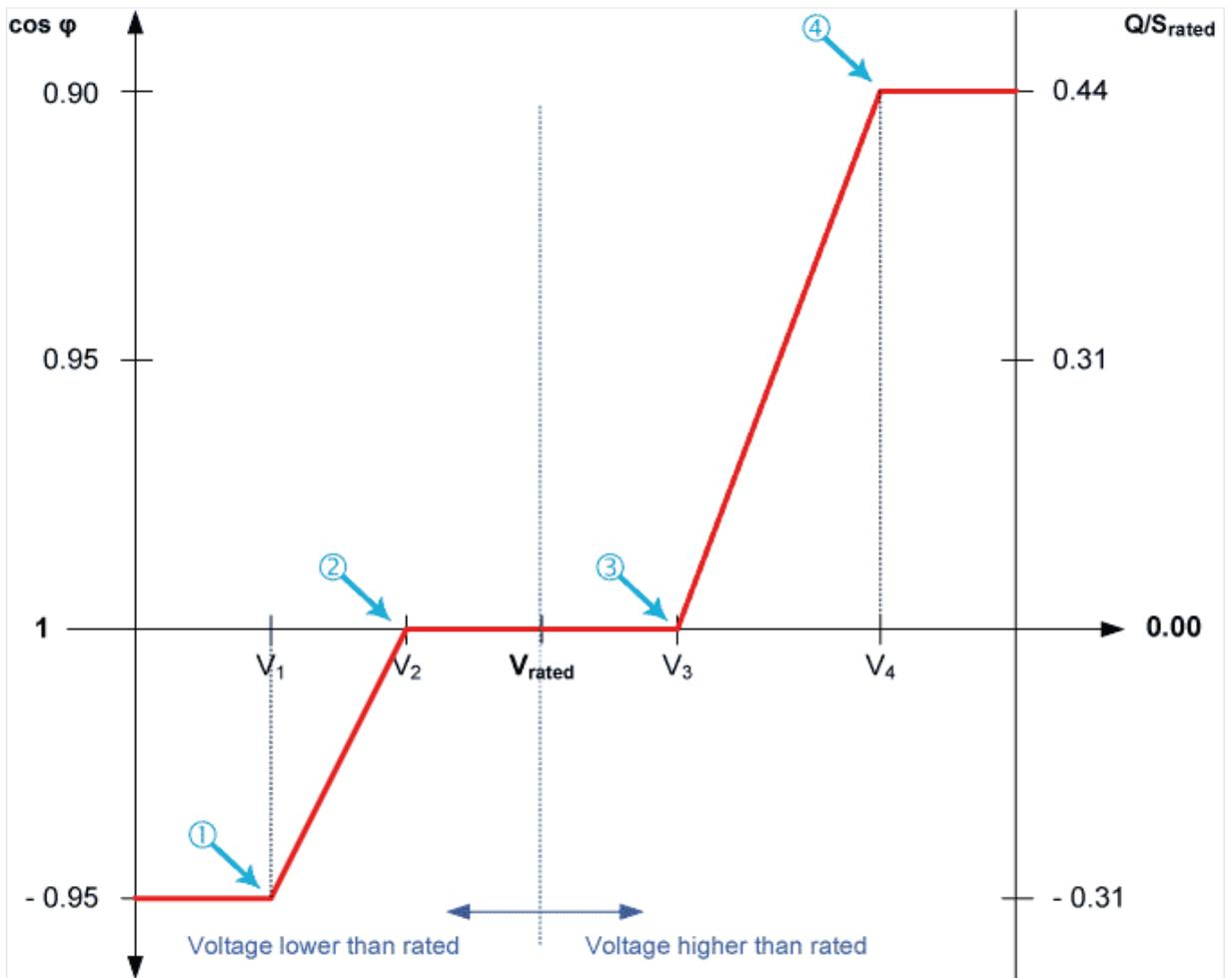
Fig. 165: Power factor characteristic according to the relation  $Q/S$  rated over rated voltage
