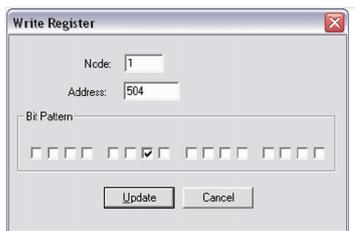
Fig. 296: Modbus - write register - shutdown command
