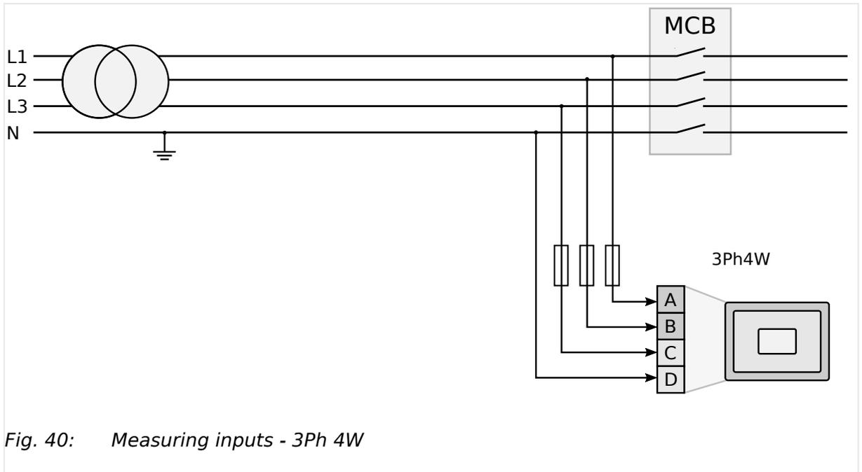
Fig. 40: Measuring inputs - 3Ph 4W
