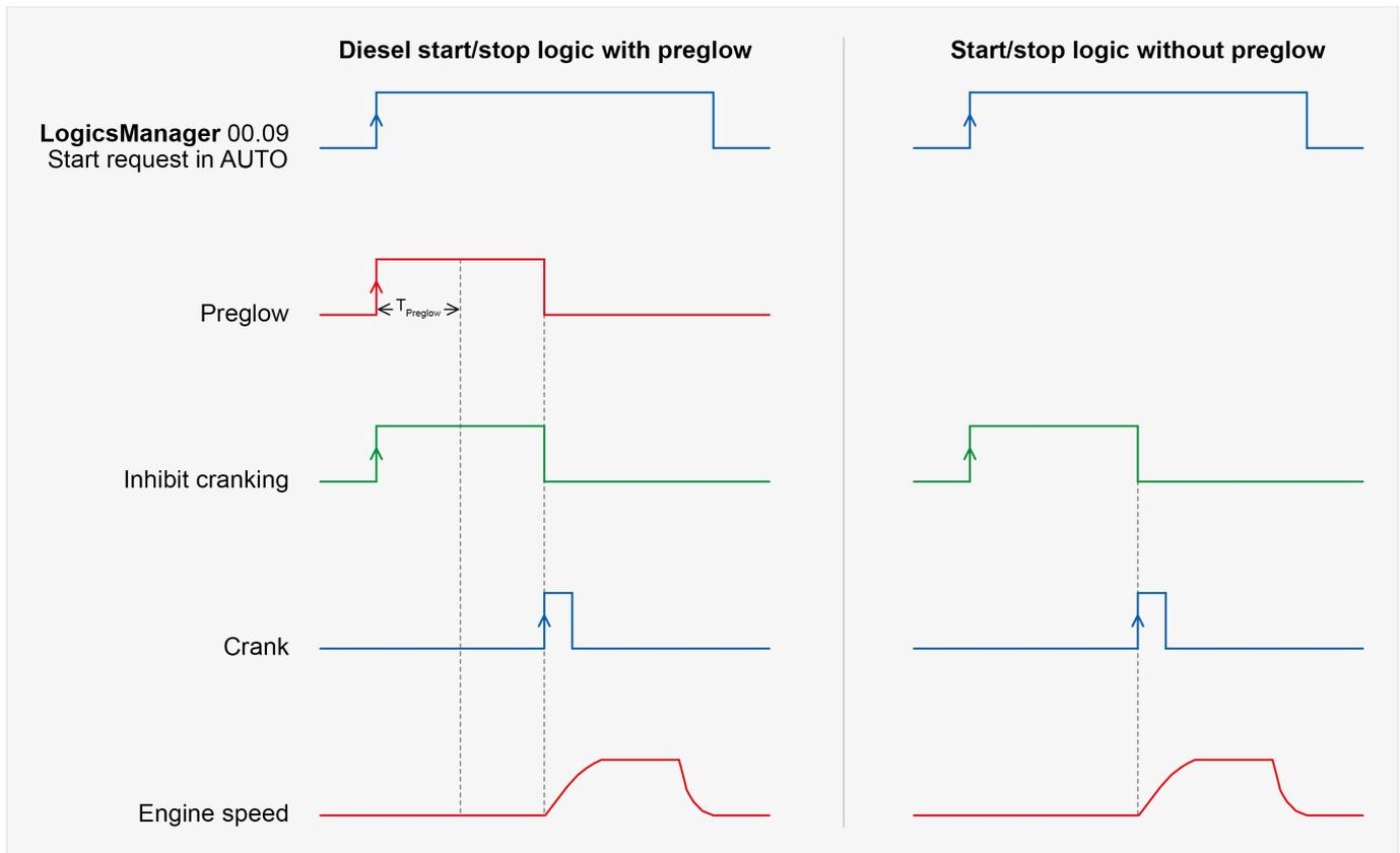
Fig. 153: Engine - start/stop logic (inhibit cranking)
