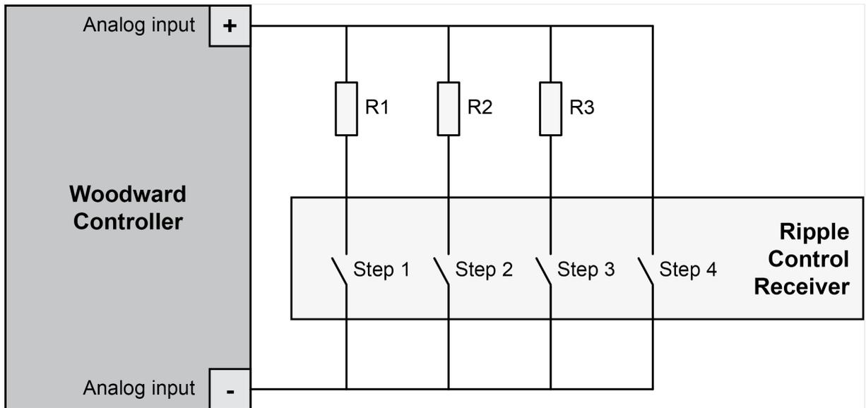
Fig. 275: Ripple control receiver wiring
