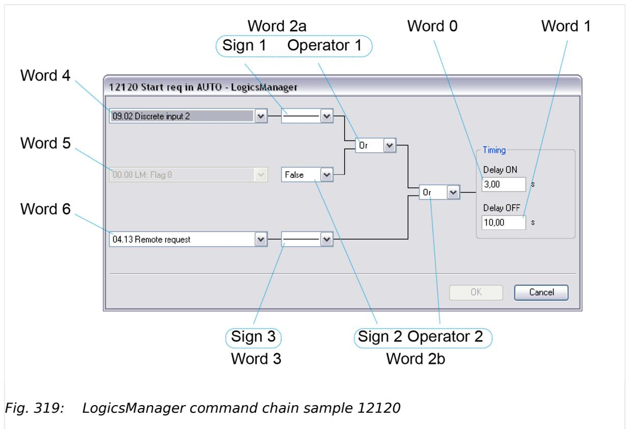
Fig. 319: LogicsManager command chain sample 12120
