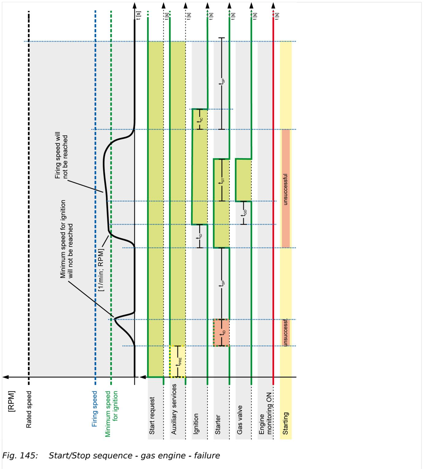
Fig. 145: Start/Stop sequence - gas engine - failure
