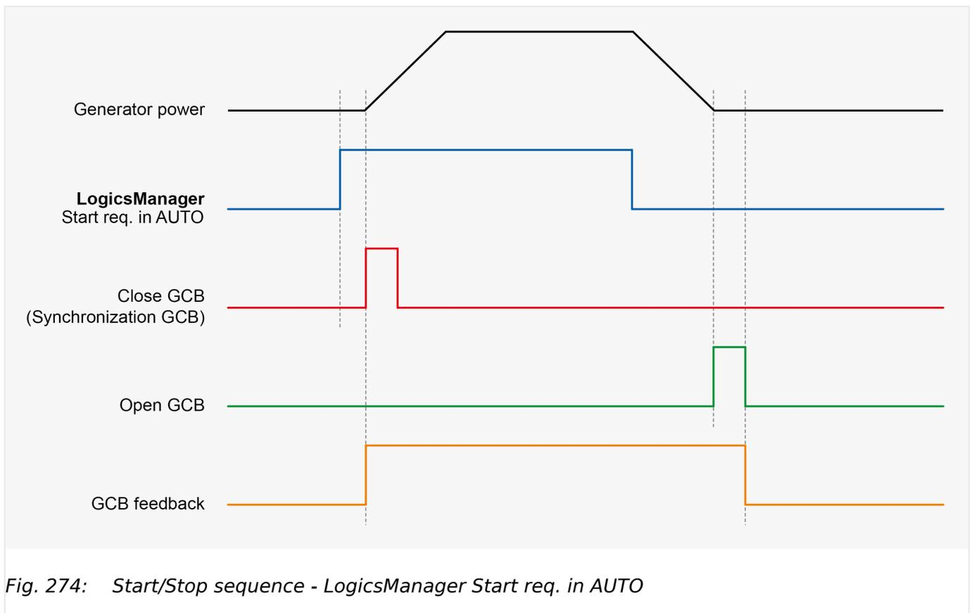
Fig. 274: Start/Stop sequence - LogicsManager Start req. in AUTO
