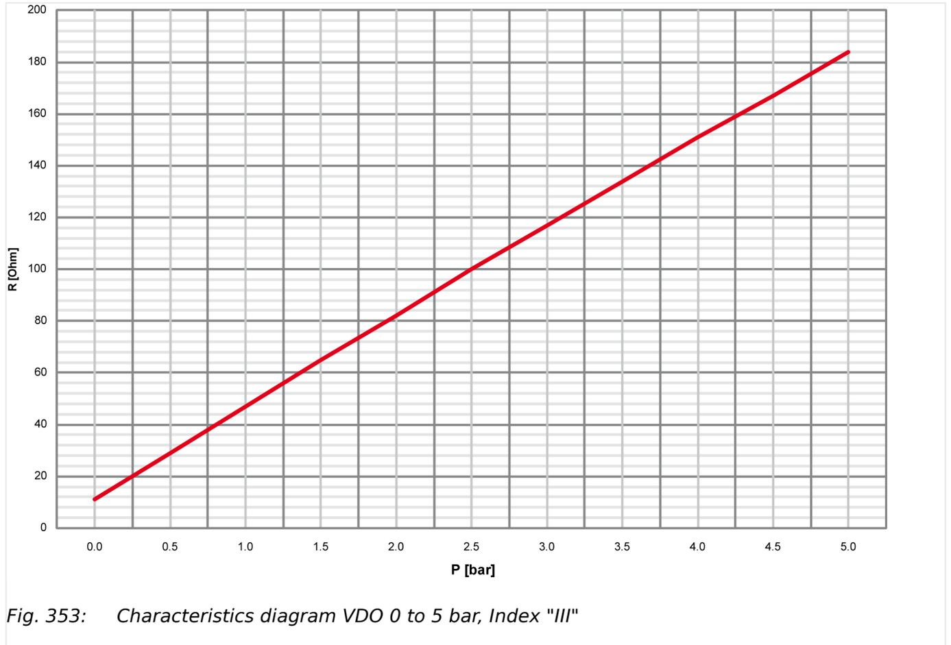
Fig. 353: Characteristics diagram VDO 0 to 5 bar, Index "III"
