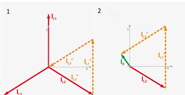
Fig. 193: Generator ground fault - calculation
