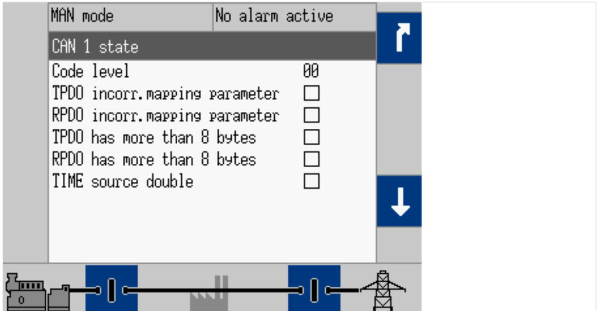
Fig. 118: CAN 1 state screen (example)
