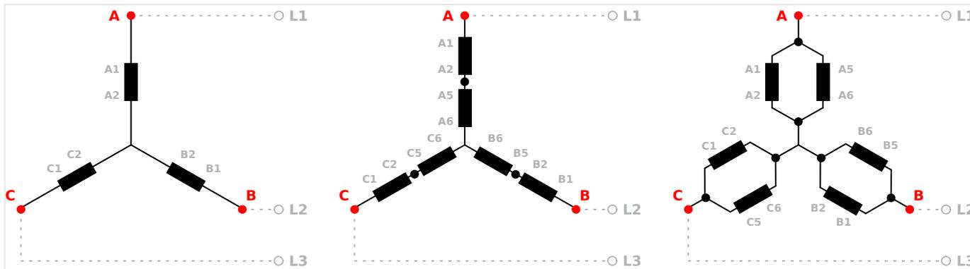
Fig. 26: Generator windings - 3Ph 4W OD
