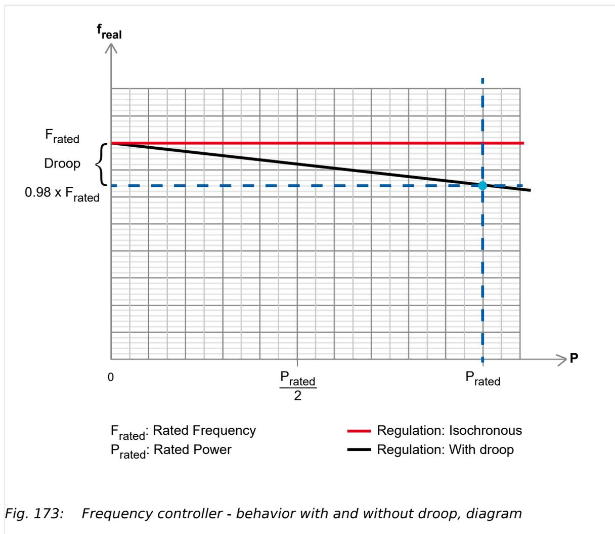
The resulting frequency setpoint is calculated as follows:  $F'_{\text{Set}} = F_{\text{Set}} - (P_{\text{real}} * (F_{\text{rated}} * \text{droop factor}) / P_{\text{rated}})$
