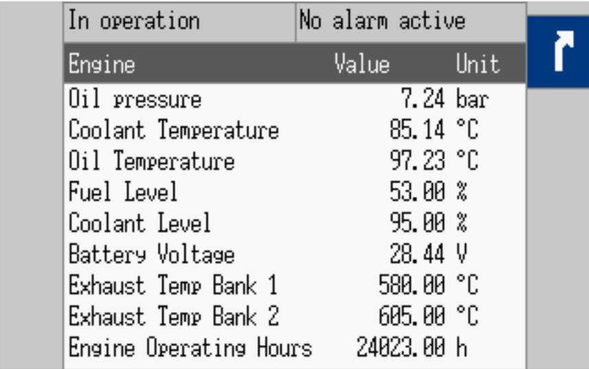
Fig. 132: Customer Screen sample: a set of interesting Engine values
