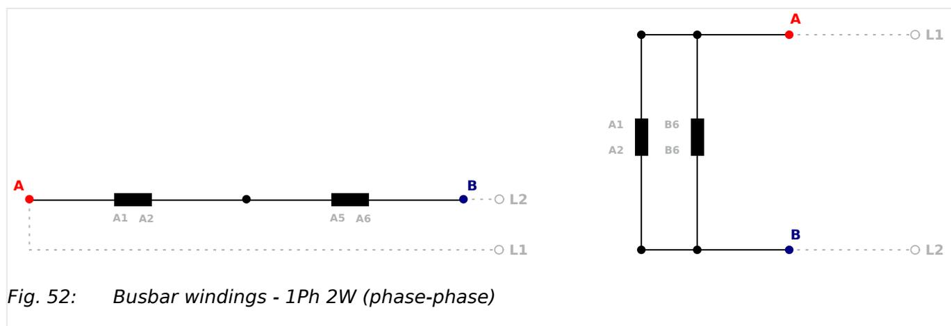
Fig. 52: Busbar windings - 1Ph 2W (phase-phase)
