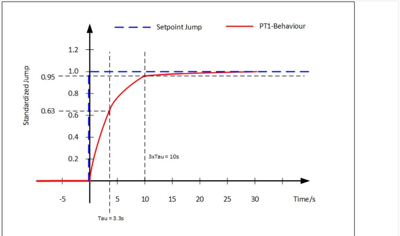
Fig. 166: Setpoint Jump (standardized with height 1) and the resulting PT1 setpoint
