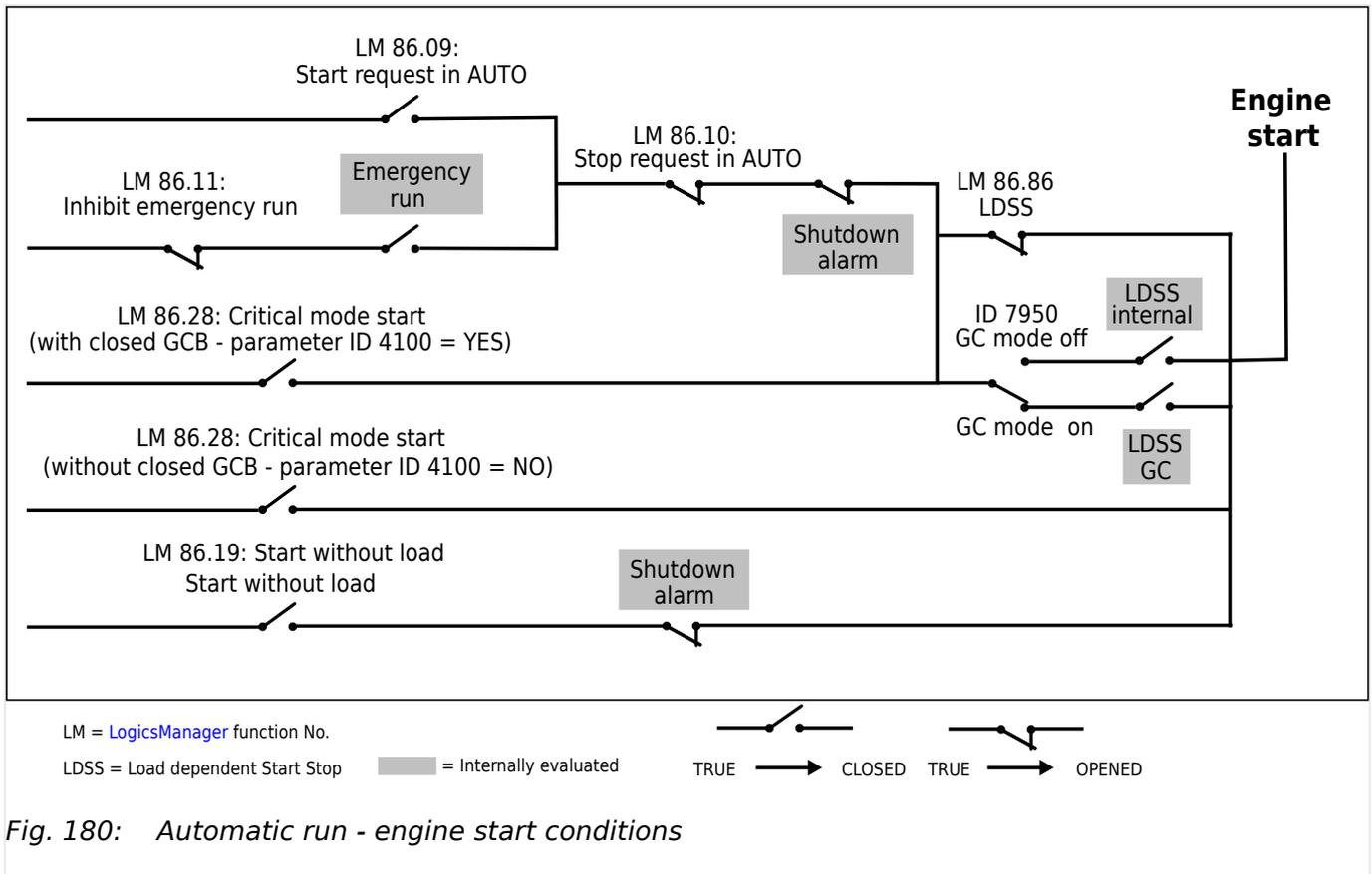
Fig. 180: Automatic run - engine start conditions
