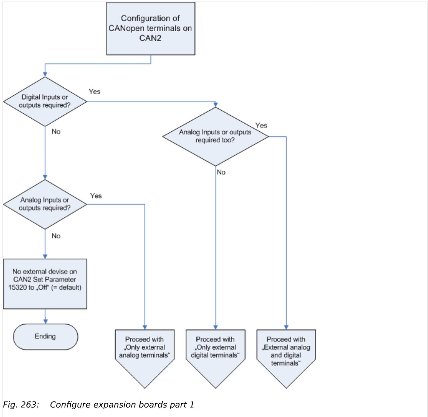
Fig. 263: Configure expansion boards part 1
