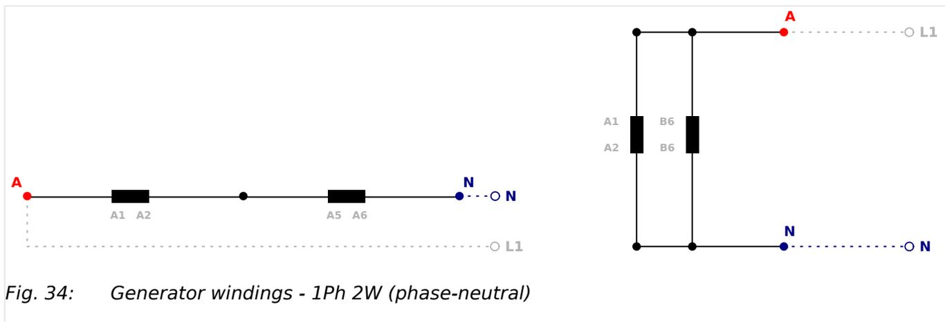
Fig. 34: Generator windings - 1Ph 2W (phase-neutral)
