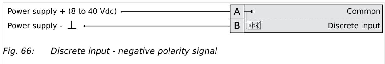
Fig. 66: Discrete input - negative polarity signal
