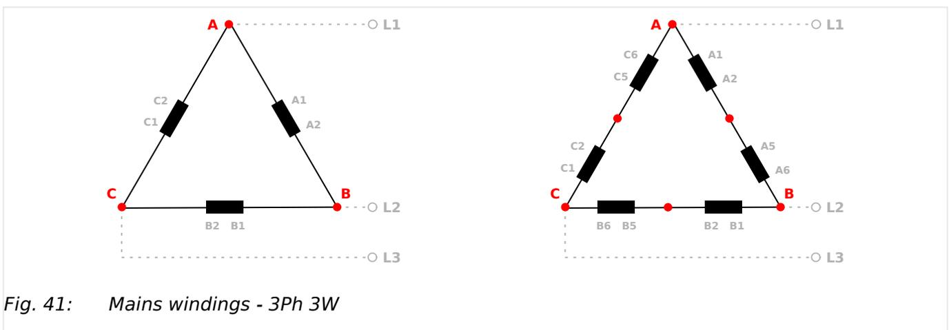
Fig. 41: Mains windings - 3Ph 3W
