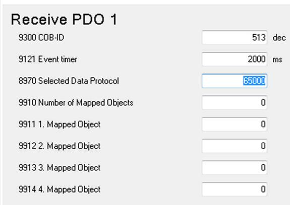
Fig. 253: RPDO configuration for the first IKD (example ToolKit)
