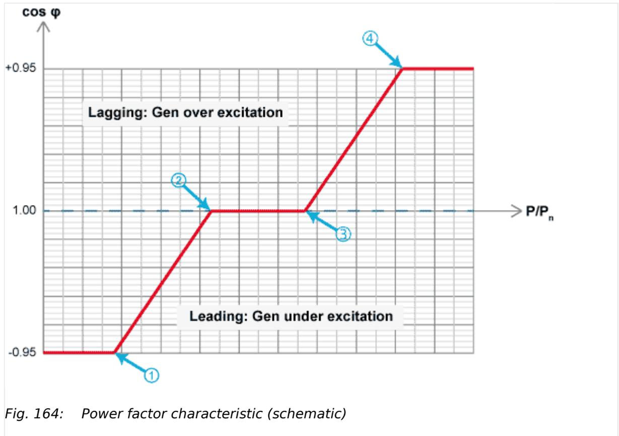
Fig. 164: Power factor characteristic (schematic)
