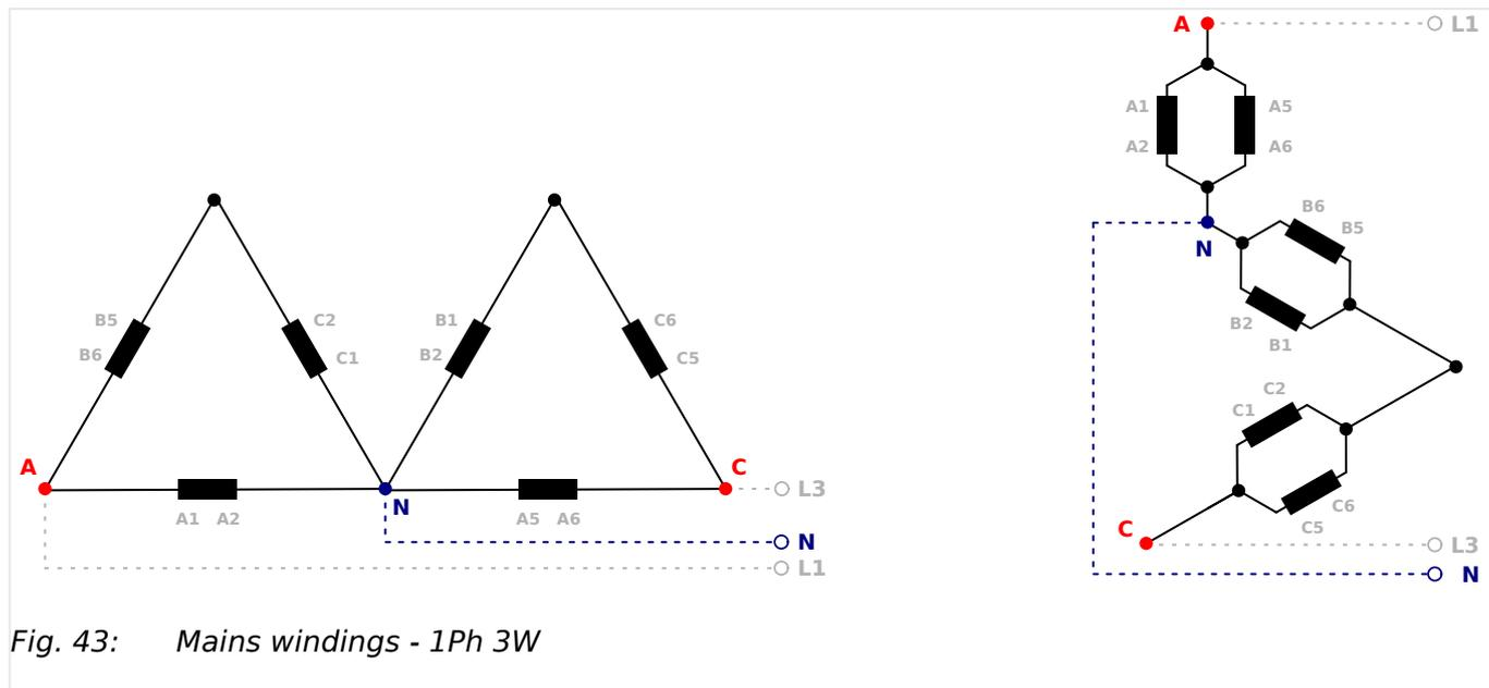
Fig. 43: Mains windings - 1Ph 3W
