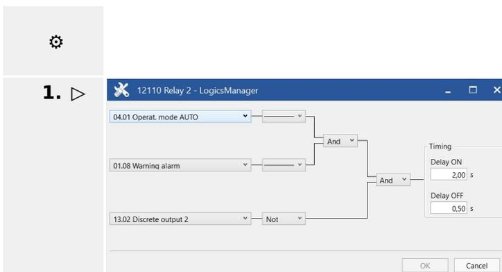
Fig. 235: LogicsManager function "Relay 2"
