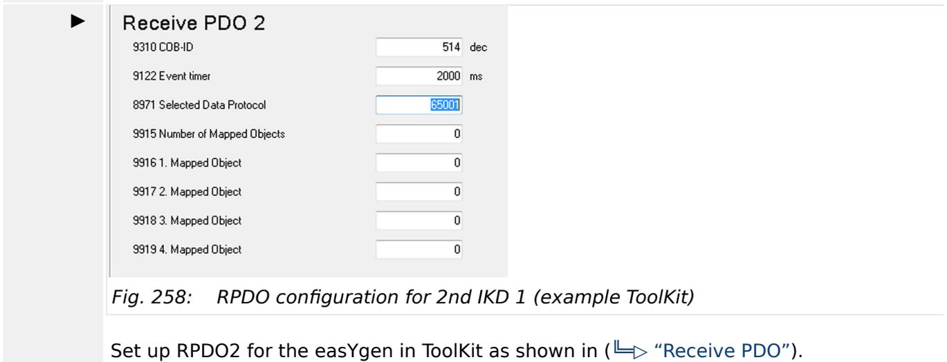
Fig. 258: RPDO configuration for 2nd IKD 1 (example ToolKit)
