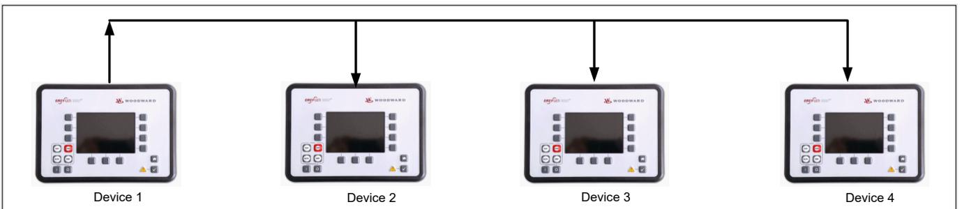
Fig. 227: Device 1 sends data to device 2, 3 and 4
