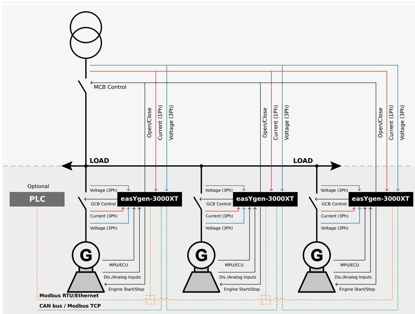
Fig. 220: Multiple genset application (schematic)
