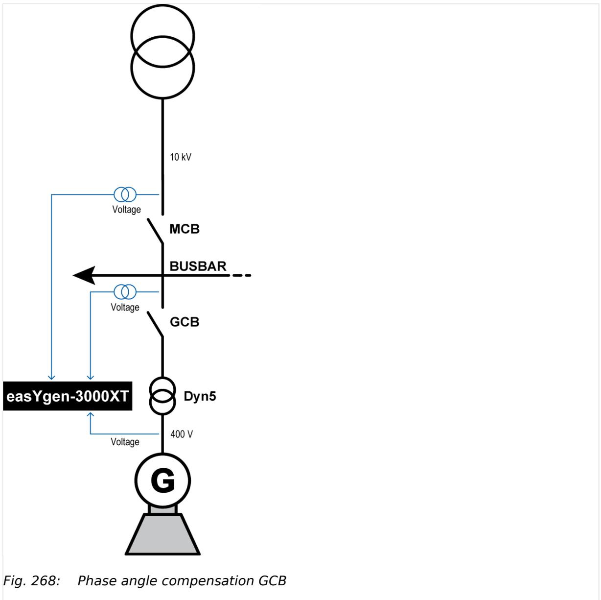
Fig. 268: Phase angle compensation GCB
