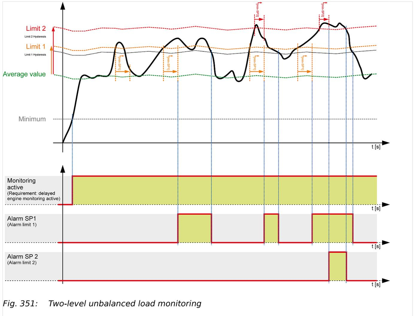
Fig. 351: Two-level unbalanced load monitoring
