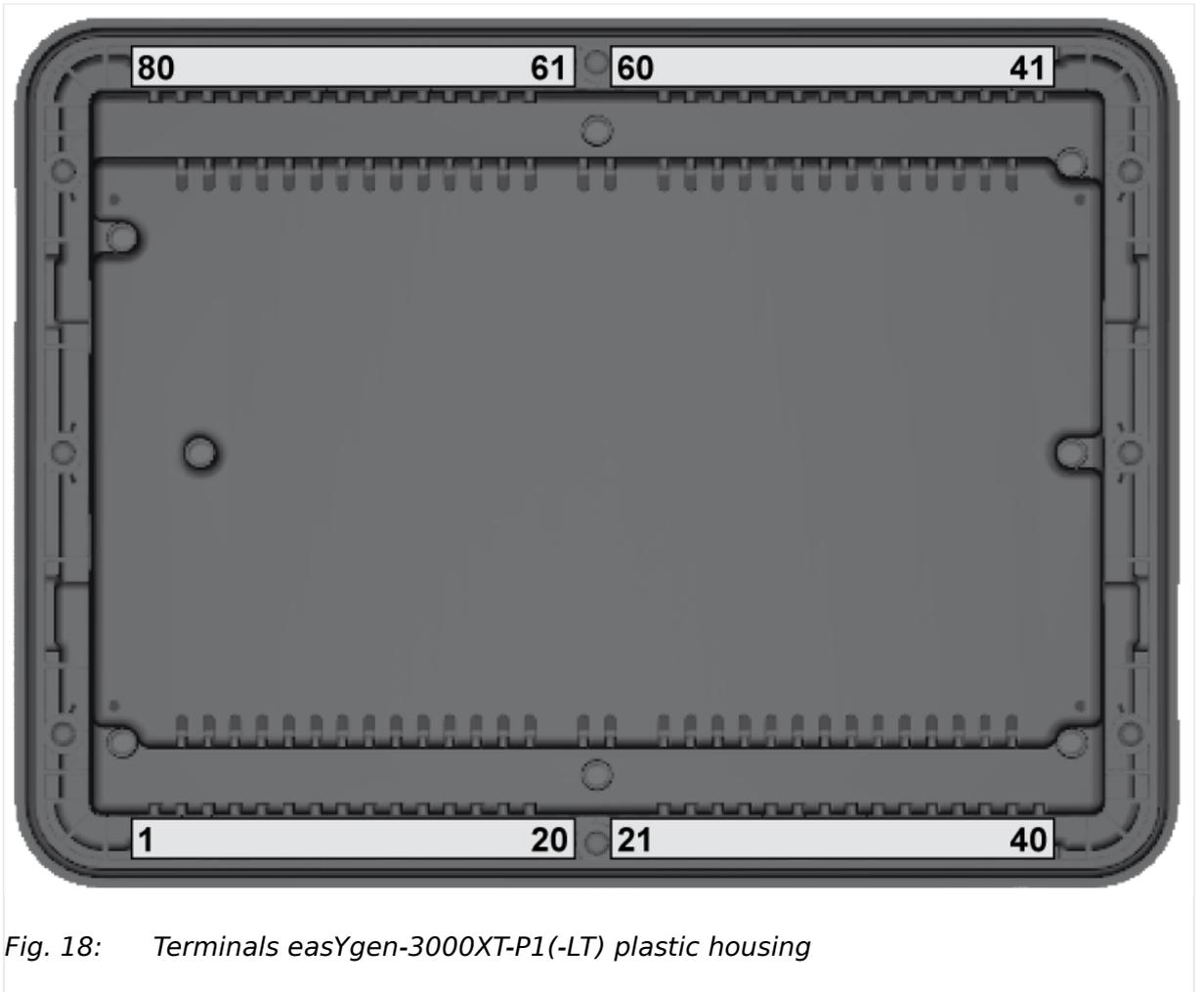
Fig. 18: Terminals easYgen-3000XT-P1(-LT) plastic housing
