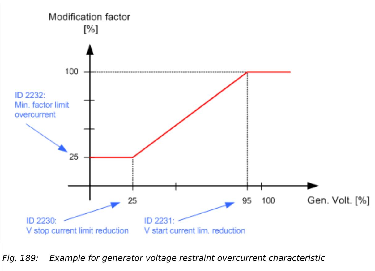
Fig. 189: Example for generator voltage restraint overcurrent characteristic
