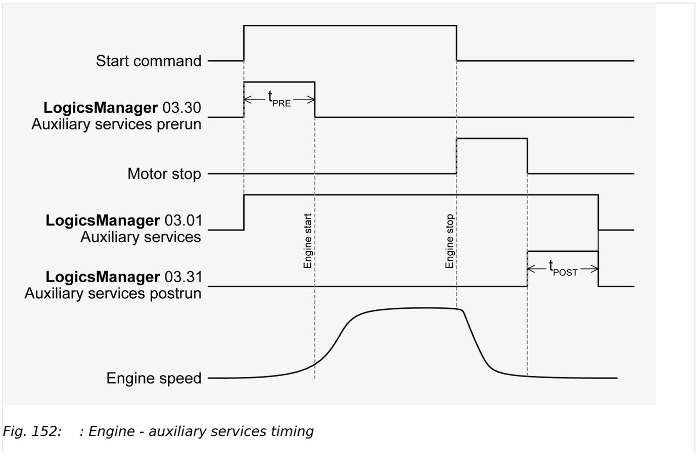
Fig. 152: : Engine - auxiliary services timing
