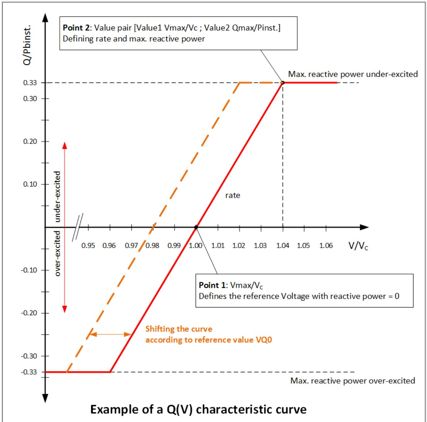
Fig. 168: EGXT\_Example\_of\_a\_Q(V)\_characteristic
