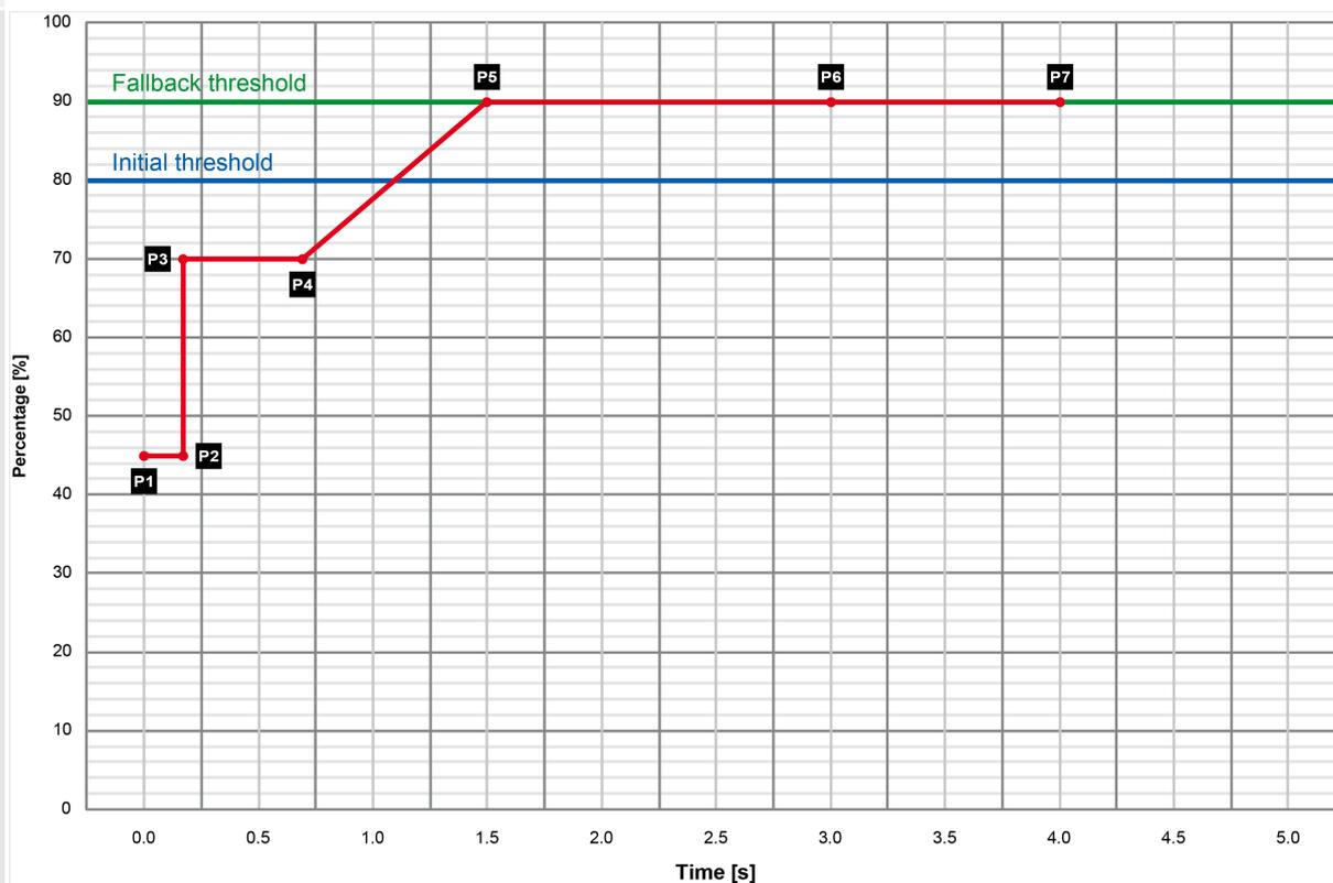
Fig. 198: Time-dependent voltage monitoring curve
