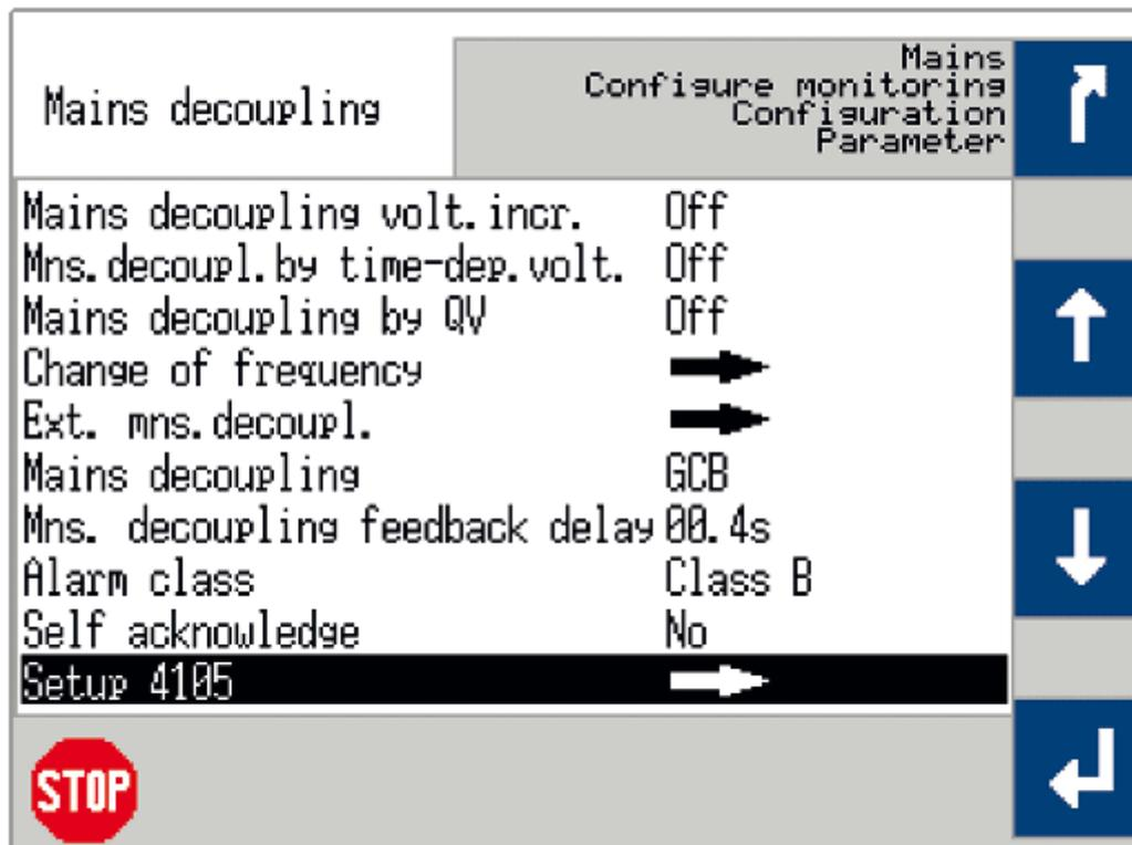
Fig. 197: Select mains decoupling 4105
