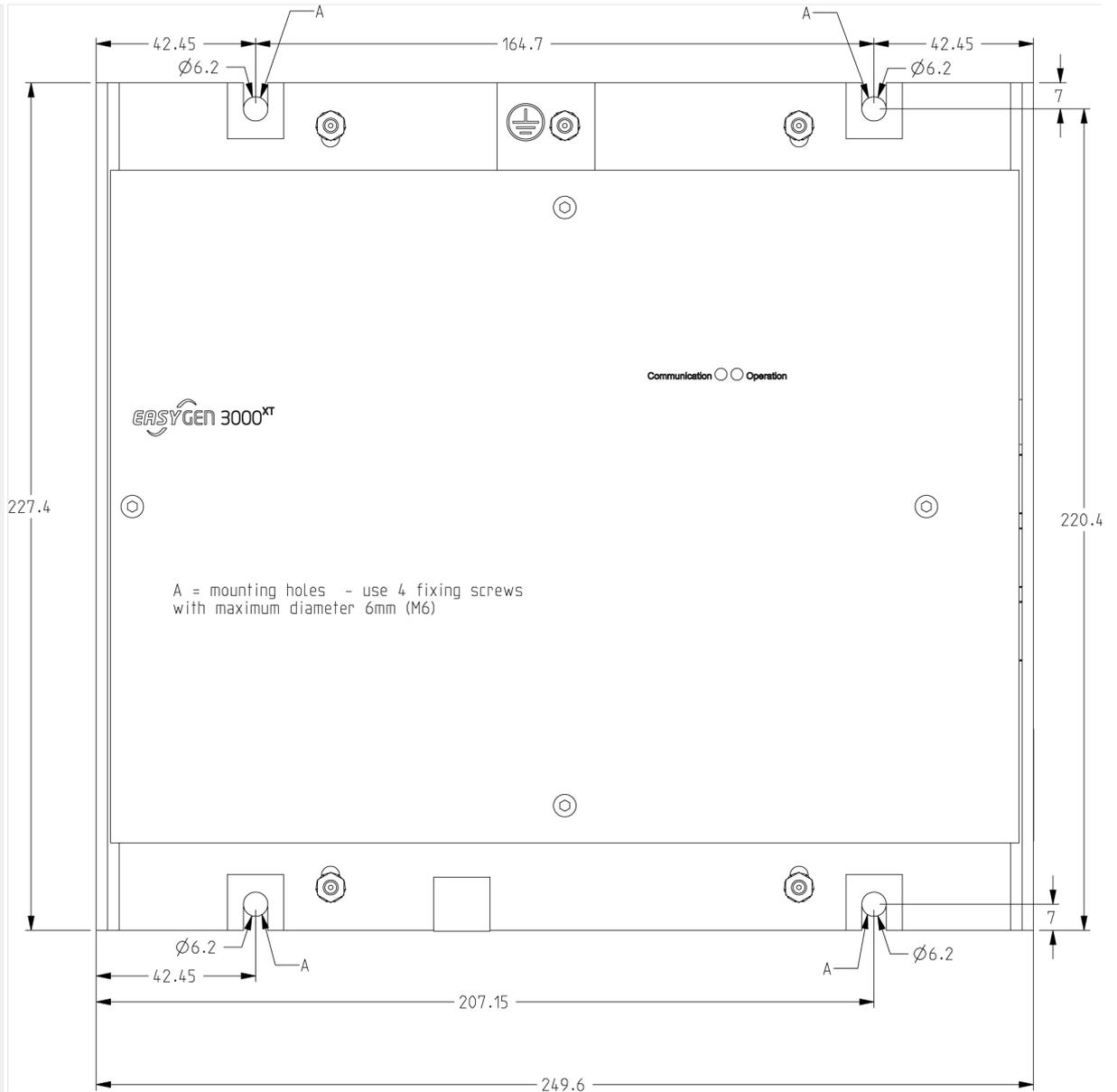
Fig. 9: Sheet metal housing - drill plan
