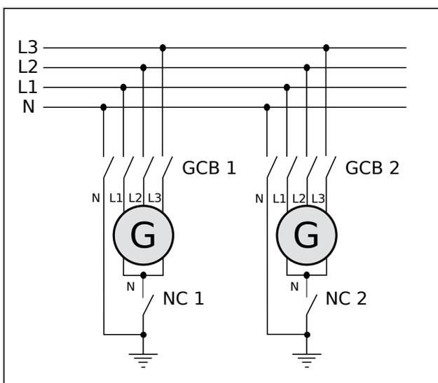
Fig. 279: Wiring neutral Interlocking: GCB 4-pole
