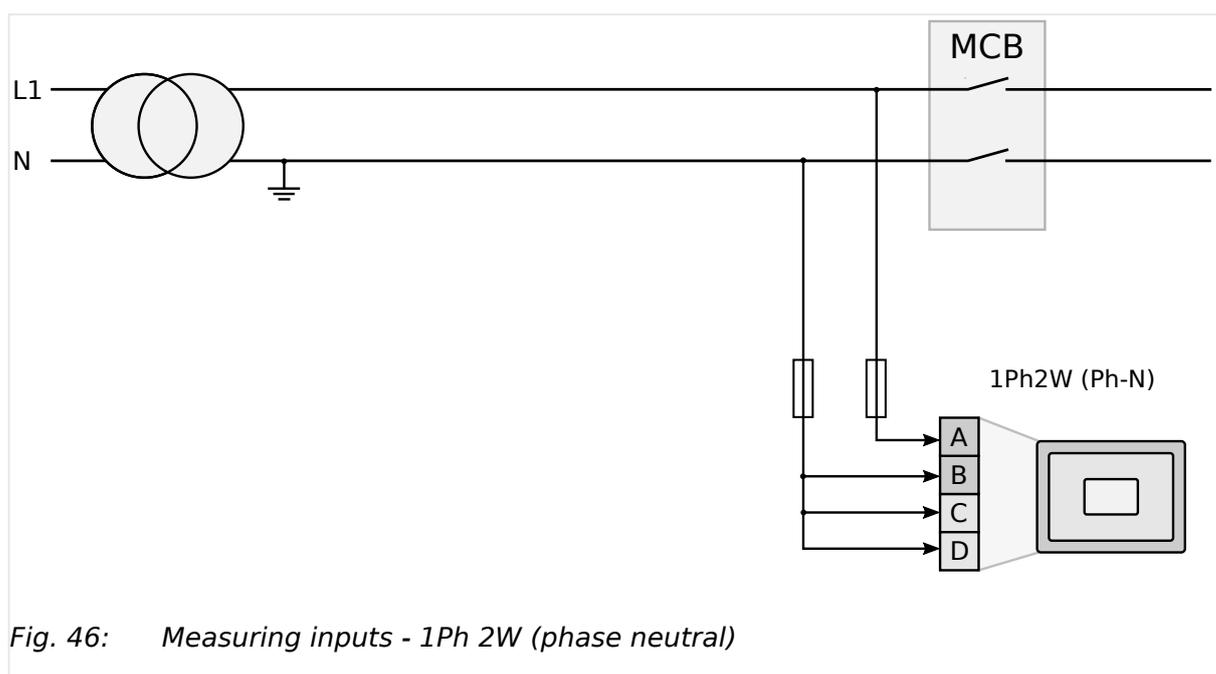
Fig. 46: Measuring inputs - 1Ph 2W (phase neutral)
