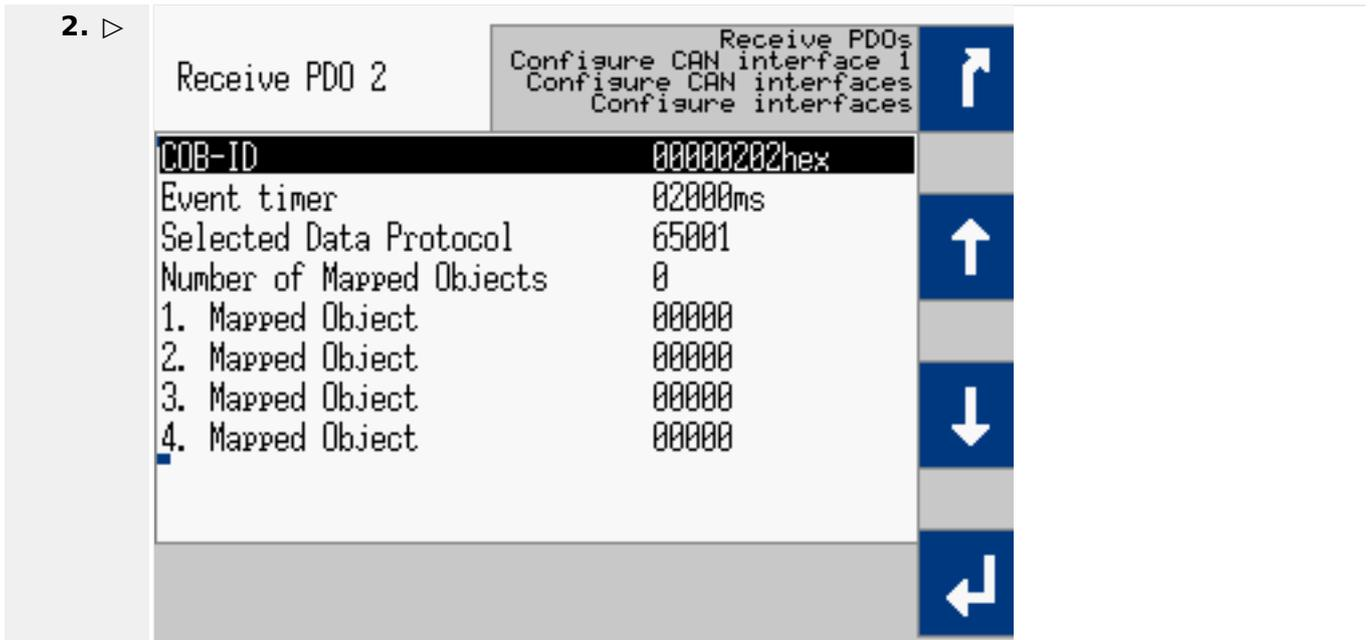
Fig. 257: RPDO configuration for 2nd IKD 1 (example HMI)
