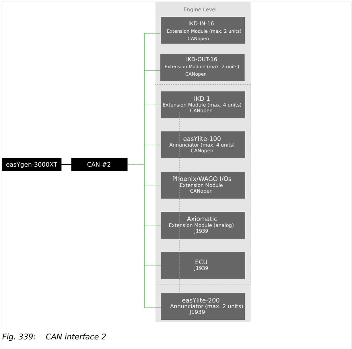
CAN interface 2 is pre-configured for several expansion units. These include the I/O expansion boards Woodward IKD 1 (or IKD-IN-16 or IKD-OUT-16), several combinations of the expansion boards of the Phoenix Inline Modular (IL) series, and the support of Wago terminals.
