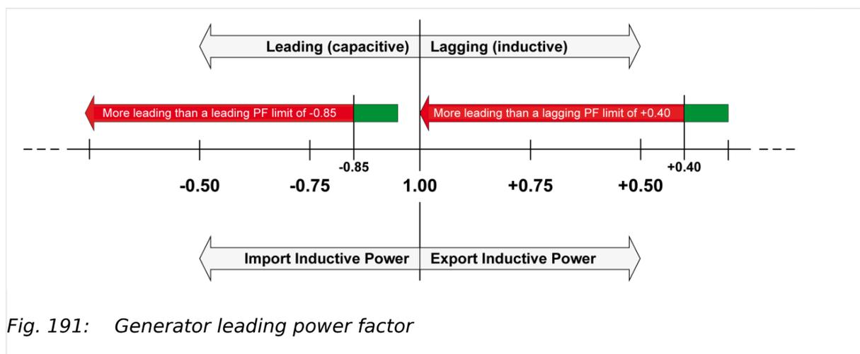
Fig. 191: Generator leading power factor
