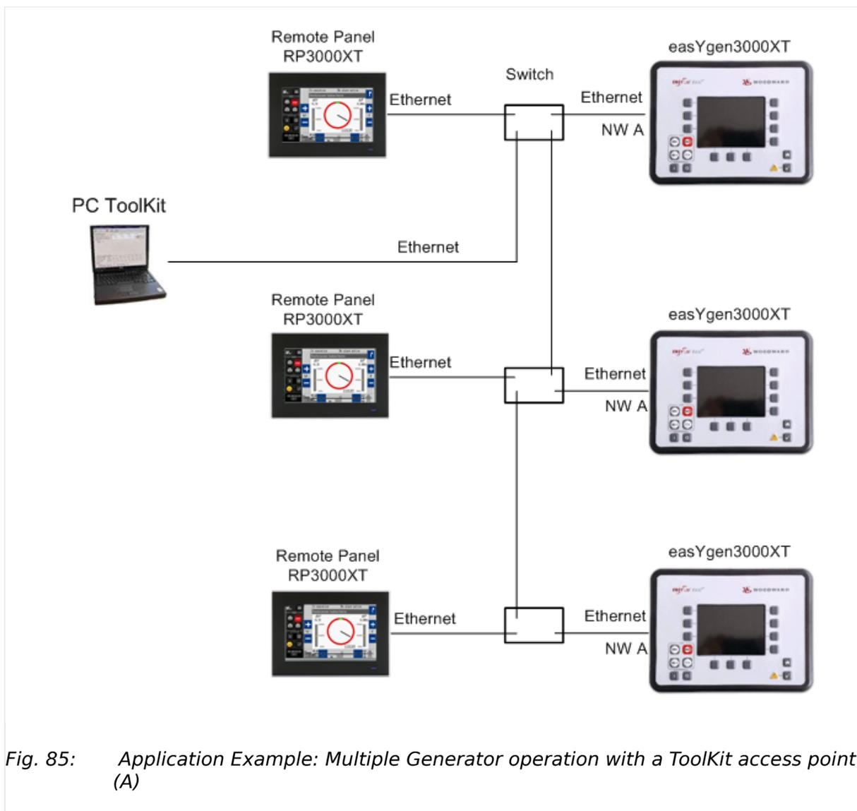
Fig. 85: Application Example: Multiple Generator operation with a ToolKit access point (A)
