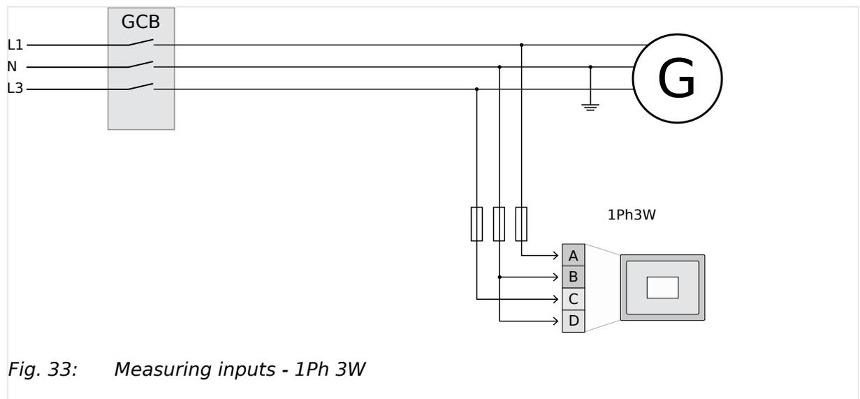
Fig. 33: Measuring inputs - 1Ph 3W
