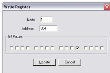
Fig. 295: Modbus - write register - external acknowledge
