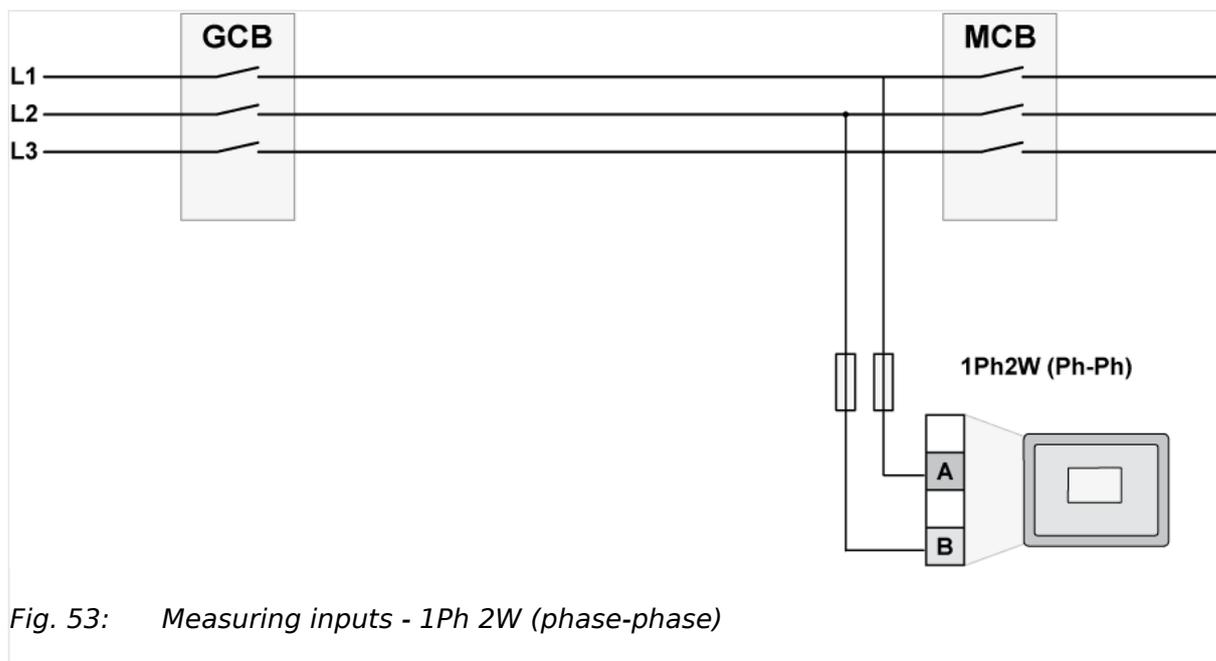
Fig. 53: Measuring inputs - 1Ph 2W (phase-phase)
