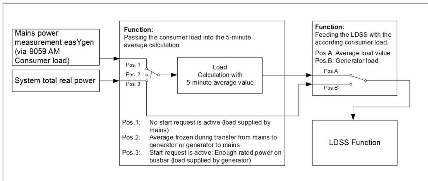
Fig. 283: Schematic of a predicted load with „internal“ source handling
