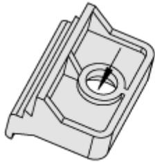
Fig. 13: Insert screws in clamps
