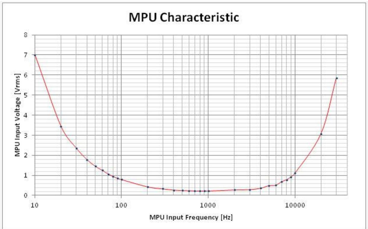
Fig. 346: MPU - characteristic
