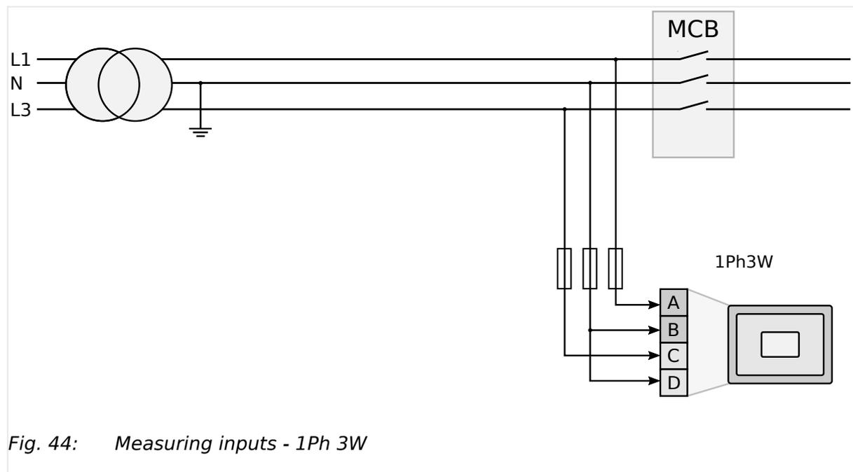
Fig. 44: Measuring inputs - 1Ph 3W
