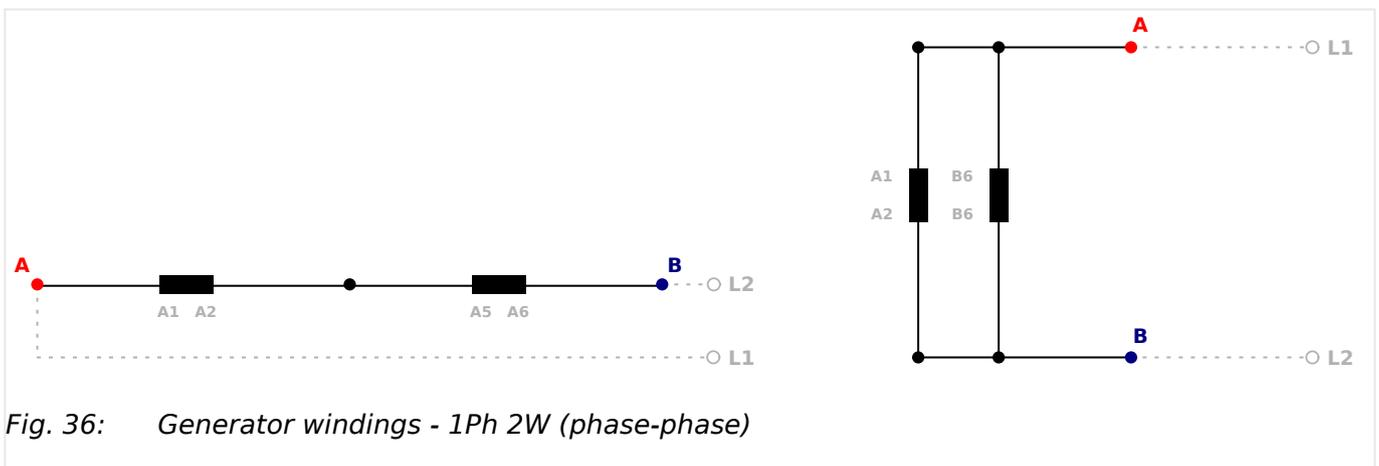
Fig. 36: Generator windings - 1Ph 2W (phase-phase)
