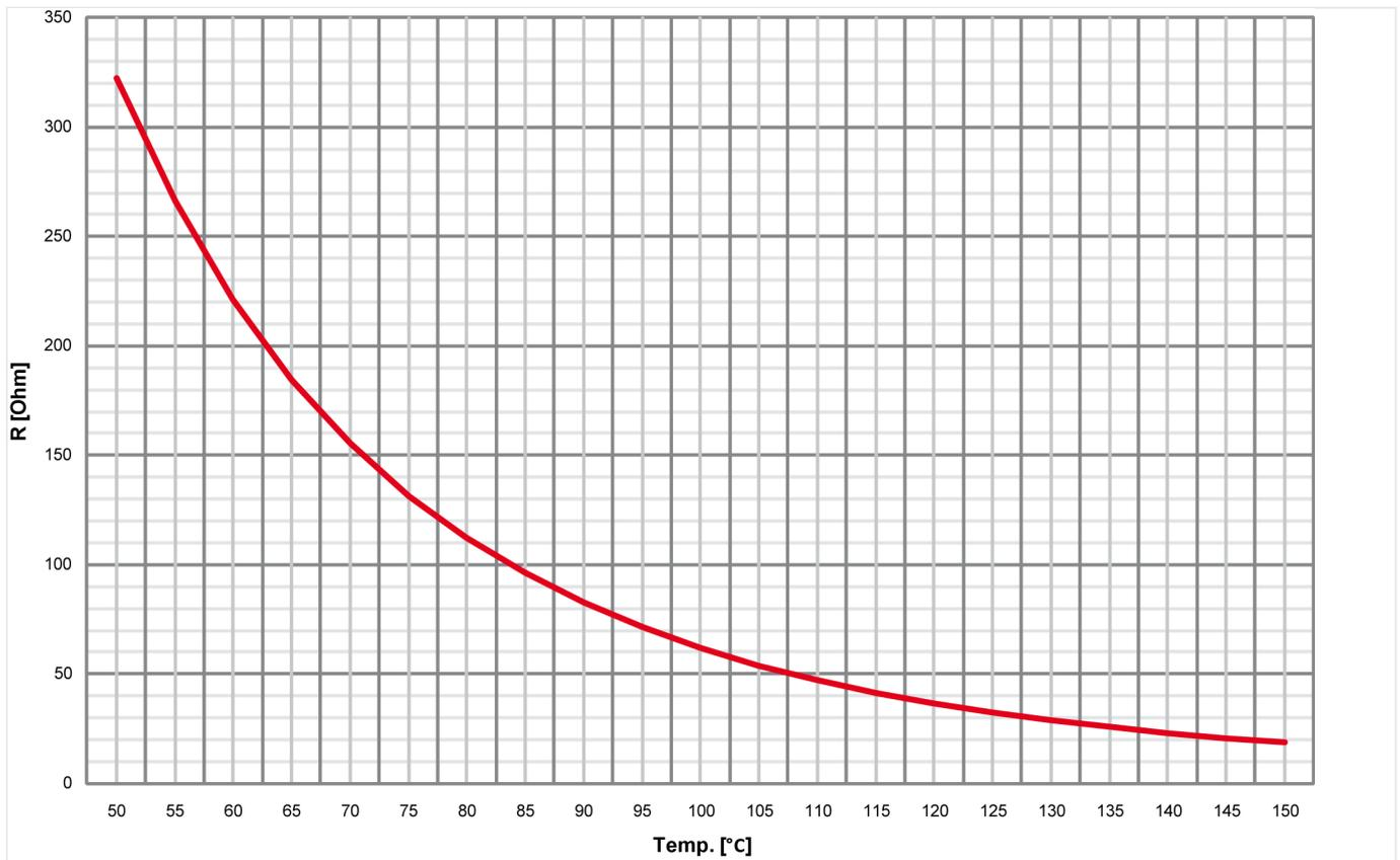
Fig. 357: Characteristics diagram VDO 50 to 150 °C - detail, Index "92-027-006"
