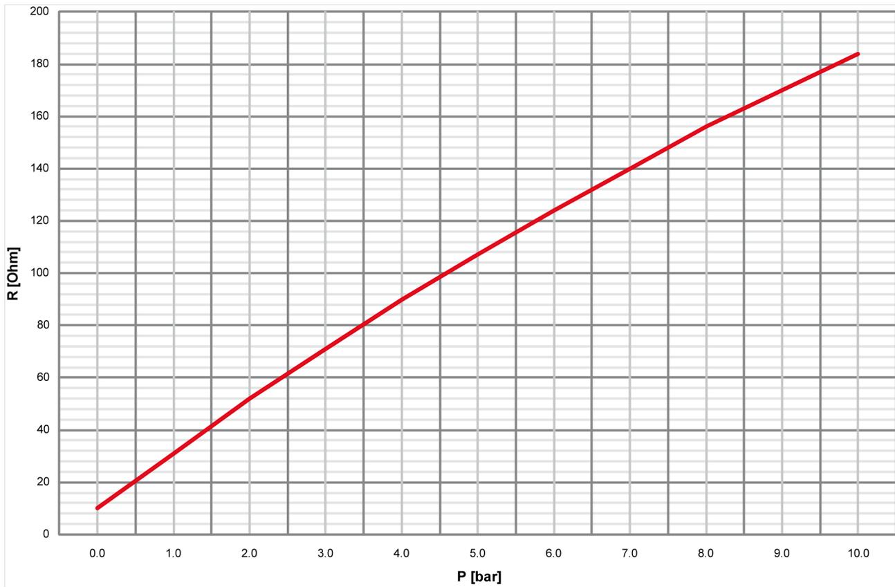
Fig. 354: Characteristics diagram VDO 0 to 10 bar, Index "IV"
