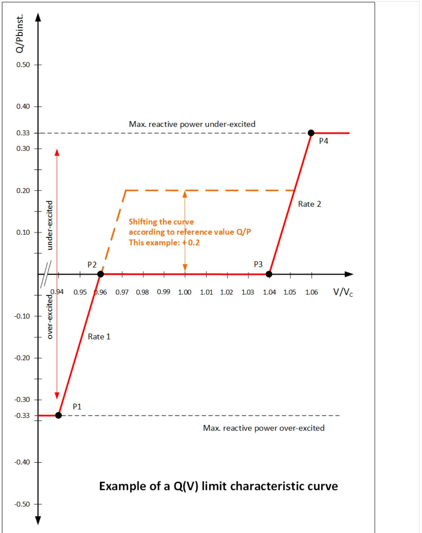
Fig. 170: Example of a Q(V) limit characteristic
