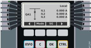
The new position of the switchgear device is shown on the display (as soon as it has been reached according to the feedback of the position indication, or after the configured switching time has elapsed).
