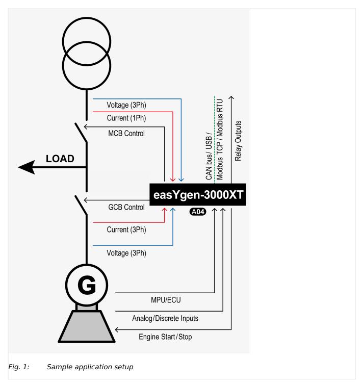
A typical application mode for the control unit is the use for mains parallel operation application.
